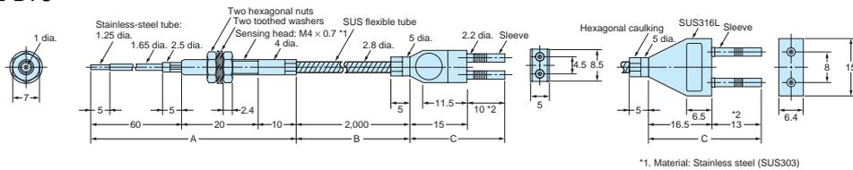
Note: The maximum allowable temperatures for sections A, B, and C are 400°C, 300°C, and 110°C, respectively. The section inserted into the Amplifier Unit (indicated by \*2), however, must stay within the Amplifier Unit's operating temperature range.
