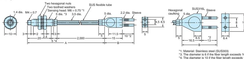
Note: The maximum allowable temperatures for sections A and B are 350°C and 110°C, respectively. The section inserted into the Amplifier Unit (indicated by \*2), however, must stay within the Amplifier Unit's operating temperature range.
