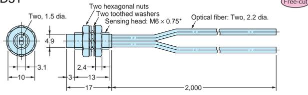
Note: The maximum allowable temperature is 150°C. The maximum allowable temperature for continuous operation is 130°C.
