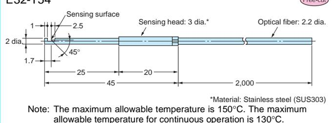
Note: The maximum allowable temperature is 150°C. The maximum allowable temperature for continuous operation is 130°C.
