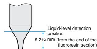
The liquid-level detection position varies with the surface tension of the liquid and the degree of wetness at the Fiber Unit's detection position.
