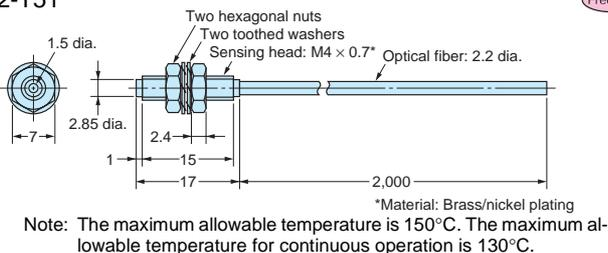
Note: The maximum allowable temperature is 150°C. The maximum allowable temperature for continuous operation is 130°C.
