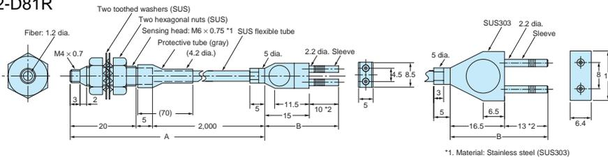
Note: The maximum allowable temperatures for sections A and B are 200°C and 110°C, respectively. The section inserted into the Amplifier Unit (indicated by \*2), however, must stay within the Amplifier Unit's operating temperature range.
