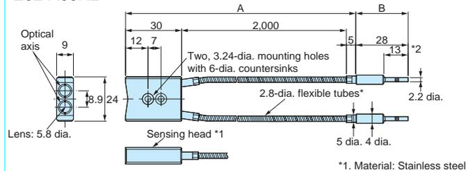
Note: The maximum allowable temperatures for sections A and B are 300°C and 110°C, respectively. The section inserted into the Amplifier Unit (indicated by \*2), however, must stay within the Amplifier Unit's operating temperature range.
