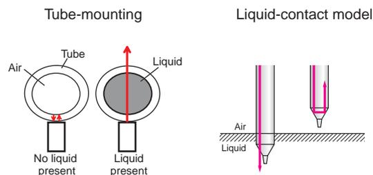
The presence/absence of liquid is detected using the refractive properties of light. More specifically, it utilizes the fact that the difference in refractive index between the air and the tip/tube is larger than the difference between the liquid and the tip/tube.
