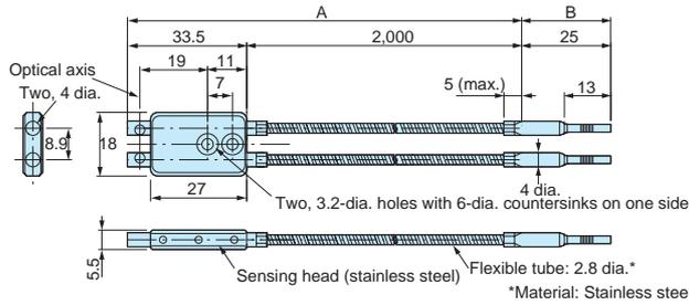
Note: The maximum allowable temperatures for sections A and B are 200°C and 110°C, respectively. The section inserted into the Amplifier Unit (indicated by \*2), however, must stay within the Amplifier Unit's operating temperature range.
