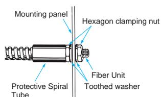
4. Use the attached saddle to secure the end cap of the Protective Spiral Tube. To secure the Protective Spiral Tube at a position other than the end cap, apply tape to the tube so that the portion becomes thicker in diameter.
