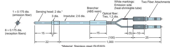
Note: The Fiber Attachment is attached with adhesive and cannot be removed.
