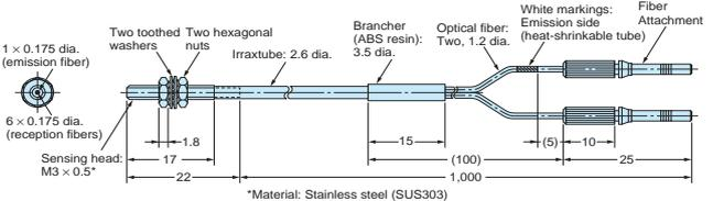
Note: The Fiber Attachment is attached with adhesive and cannot be removed.
