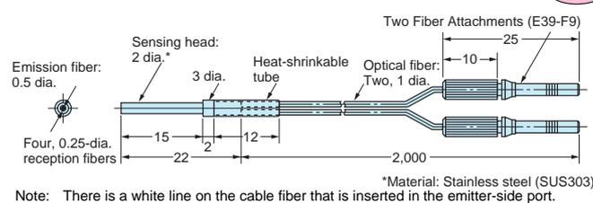
Note: There is a white line on the cable fiber that is inserted in the emitter-side port.
