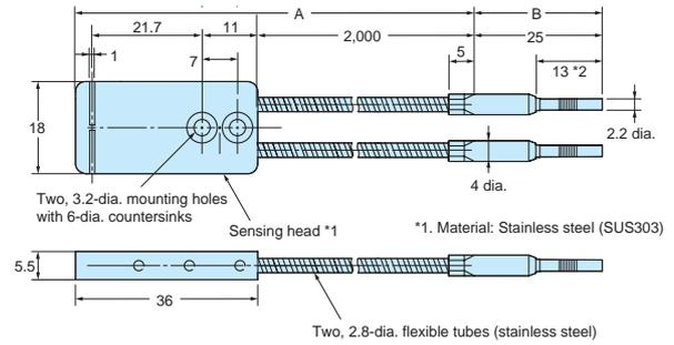
Note: The maximum allowable temperatures for sections A and B are 300°C and 110°C, respectively. The section inserted into the Amplifier Unit (indicated by \*2), however, must stay within the Amplifier Unit's operating temperature range.
