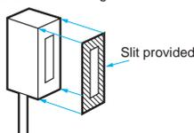
To use the slit provided, peel off the backing sheet, align it with the edges of the sensing surface, and attach it to the sensing head. Use the slit in applications where saturation occurs (i.e., changes in light intensity cannot be obtained) due to short sensing distances.
