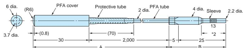
Note: The maximum allowable temperatures for sections A and B are 200°C and 110°C, respectively. The section inserted into the Amplifier Unit (indicated by \*2), however, must stay within the Amplifier Unit's operating temperature range.
