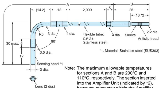
Note: The maximum allowable temperatures for sections A and B are 200°C and 110°C, respectively. The section inserted into the Amplifier Unit (indicated by \*2), however, must stay within the Amplifier Unit's operating temperature range.
