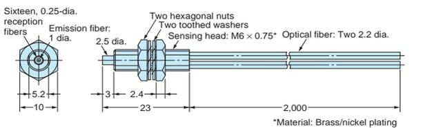
Note: There is a white line on the fiber that is inserted in the emitter-side port.
