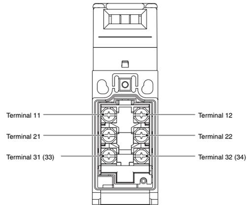
Note: The 2-conduit models have the same terminal arrangement.
