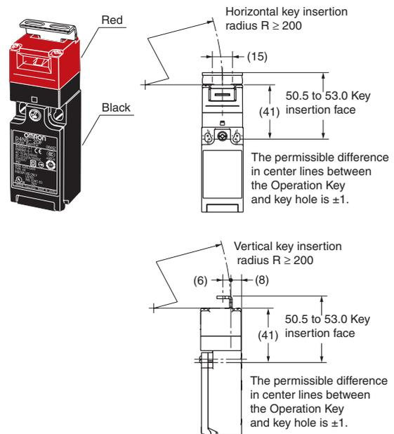
**Note:** Unless otherwise specified, a tolerance of  $\pm 0.4$  mm applies to all dimensions.
