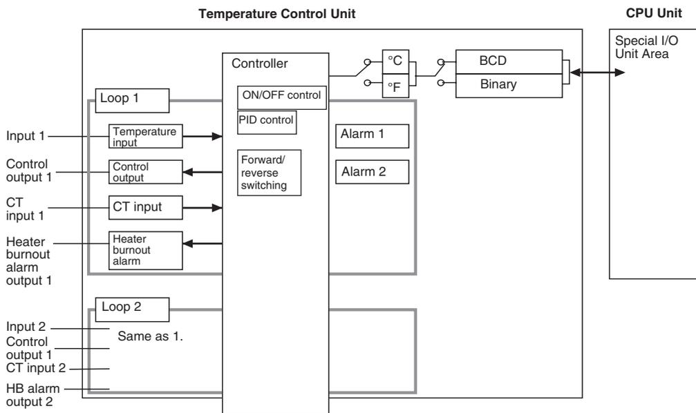
**When the Unit is used with NJ-series CPU unit**
