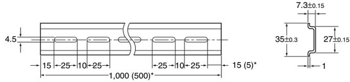
\* The dimensions given in parentheses are for the PFP-50N Socket Mounting Track.
