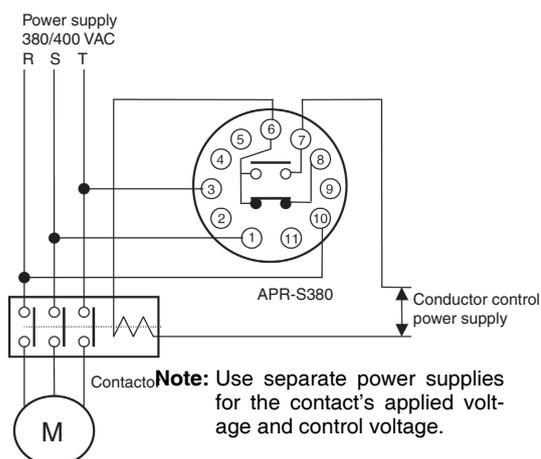
**Note:** Use separate power supplies for the contact's applied voltage and control voltage.
