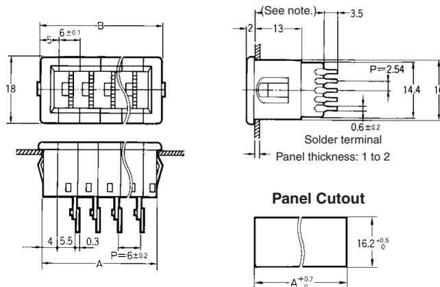
**Note:** If the output code is 06, the dimension is 19; if the output code is 07, the dimension is 31.
