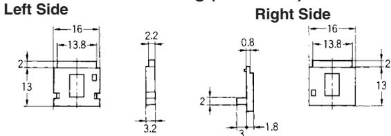
**Note:** The A7MD cannot be mounted by a screw panel or snap-in panel. Fasten the PC board after mounting the A7MD to the PC board.
