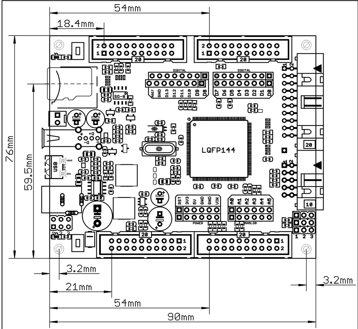
The three highest elements on the board in order from the tallest to the shortest are: capacitor C46 – 17.2mm (0.677") over the pcb; USB host connectors – 14.3mm (0.563"); capacitors C11 and C3 – 11.5mm (0.453").
