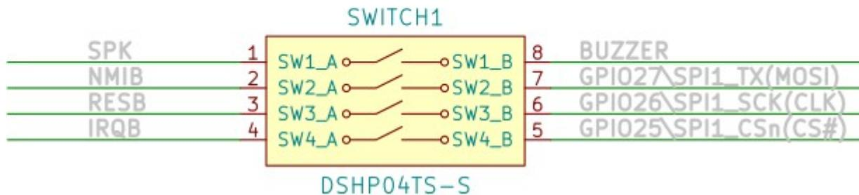
By default Neo6502 is shipped with all sections connected on the switch i.e. buzzer is enabled and all signals are wired to RP2040. This means you can't use SPI on UEXT connector if you do not disconnect these signals.
