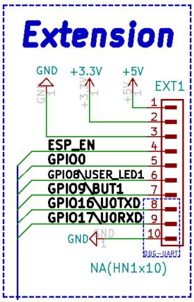
**EXT1 pin #1** is +5V pin; it is usually used as output you can also power the board from this pins **BUT ONLY IF** the USB-C is not connected! It must be regulated 5V power supply, applying more than 5V will damage the board;
