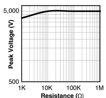
Resistors are tested in accordance with IEC61000-4-5, waveform 1.2/50μS, 10 Pulses applied. Limit of acceptance is a shift in resistance of less than 1% from the initial value. Graph data shows values equal or greater than 1KΩ.
