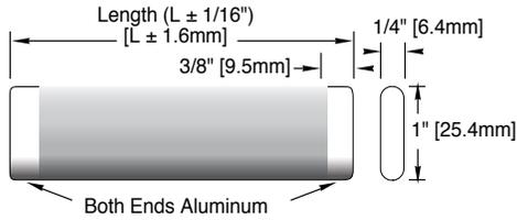
**Fig. 2 With Straight Radial Tabs (G1)**
