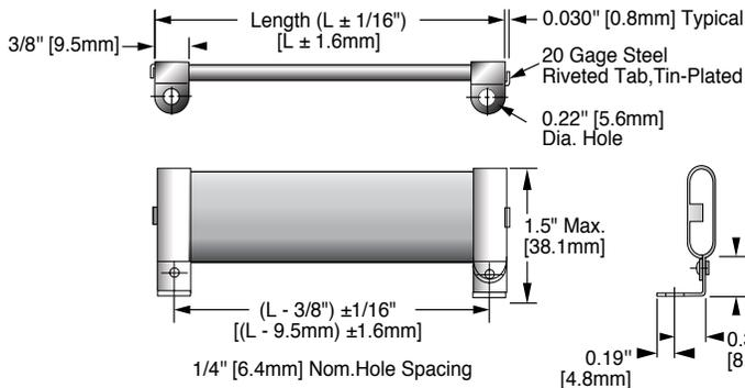
**Fig. 4 With Right Angle Radial Tabs – opposite direction – (G3)**
