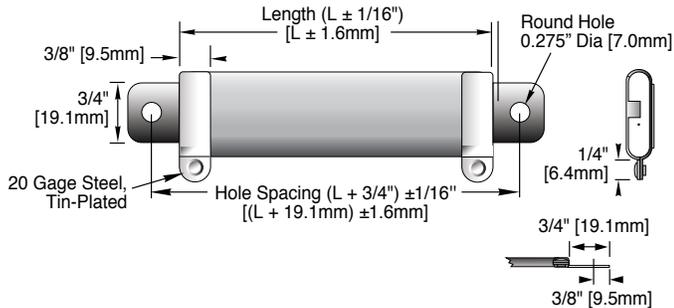
**Fig. 6 With Standoff Axial Tabs (H2)**
