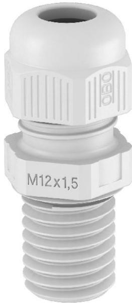
The quickest and most convenient way of providing strain relief and tightness with cable glands on junction boxes and housings is with the tried-and-trusted V-TEC VM cable glands from OBO. With the integrated sealing lip and the special OBO slat technology, protection class IP68 is achieved. Strain relief and tightness have been tested to DIN EN 62444.
