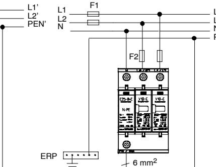
$F_1 > 125 \text{ A} \Rightarrow F_2 = 125 \text{ A}_{\text{gL}}$
