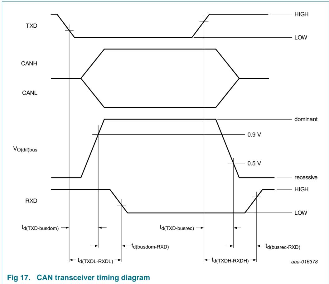
Fig 17. CAN transceiver timing diagram
