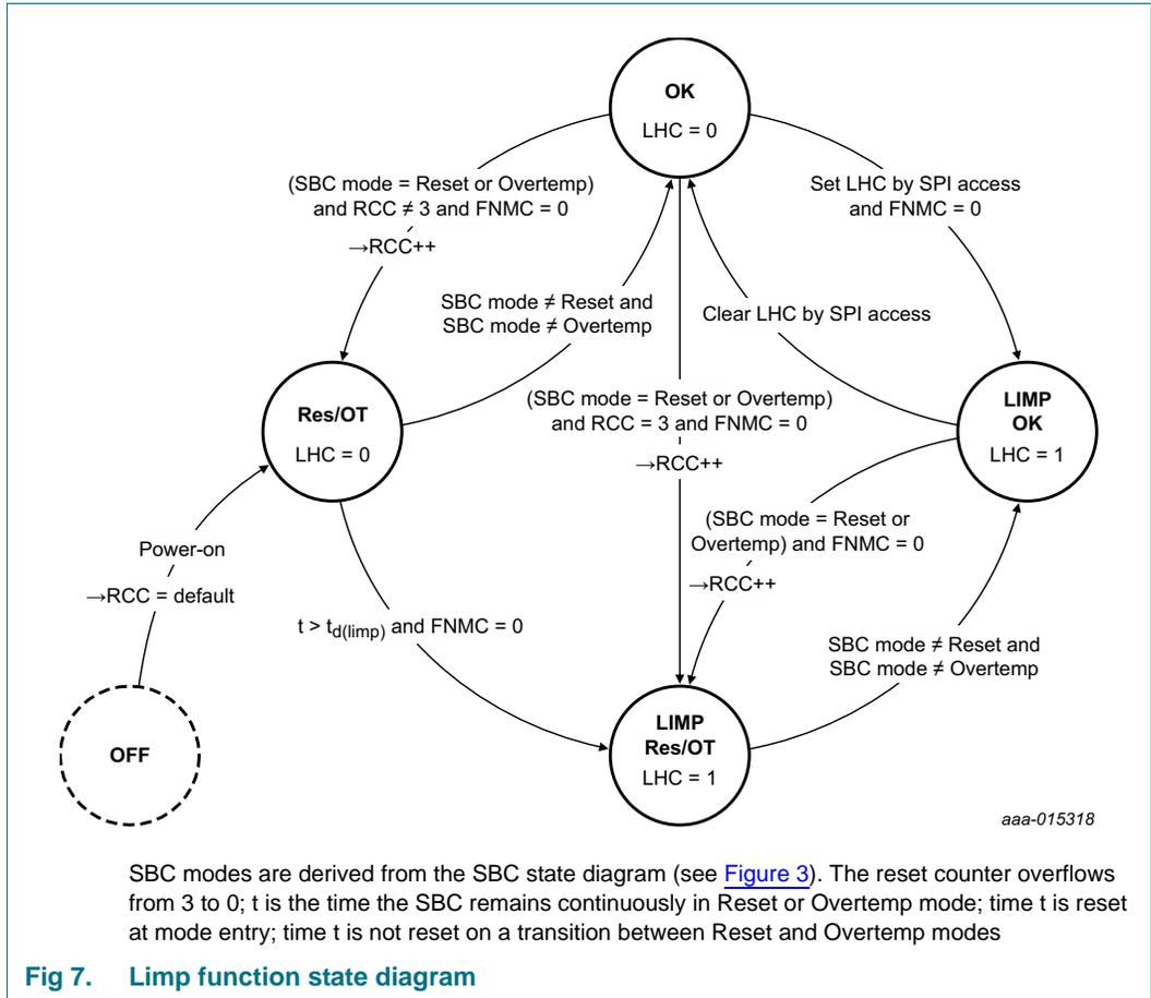
Fig 7. Limp function state diagram
