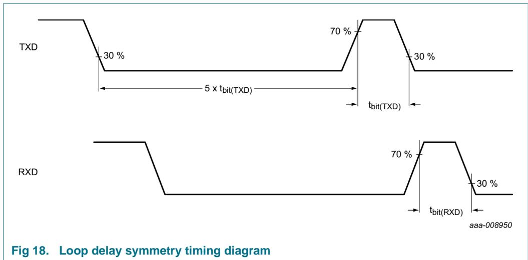
Fig 18. Loop delay symmetry timing diagram
