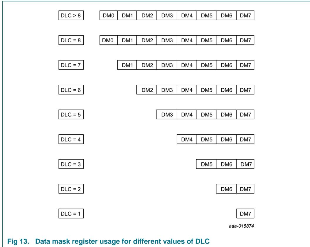
Fig 13. Data mask register usage for different values of DLC
