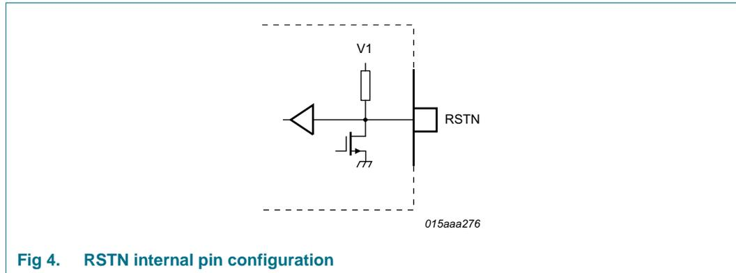
Fig 4. RSTN internal pin configuration
