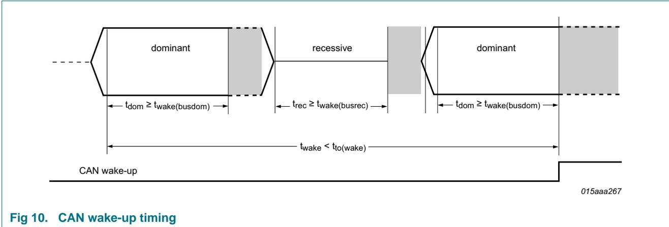
Fig 10. CAN wake-up timing
