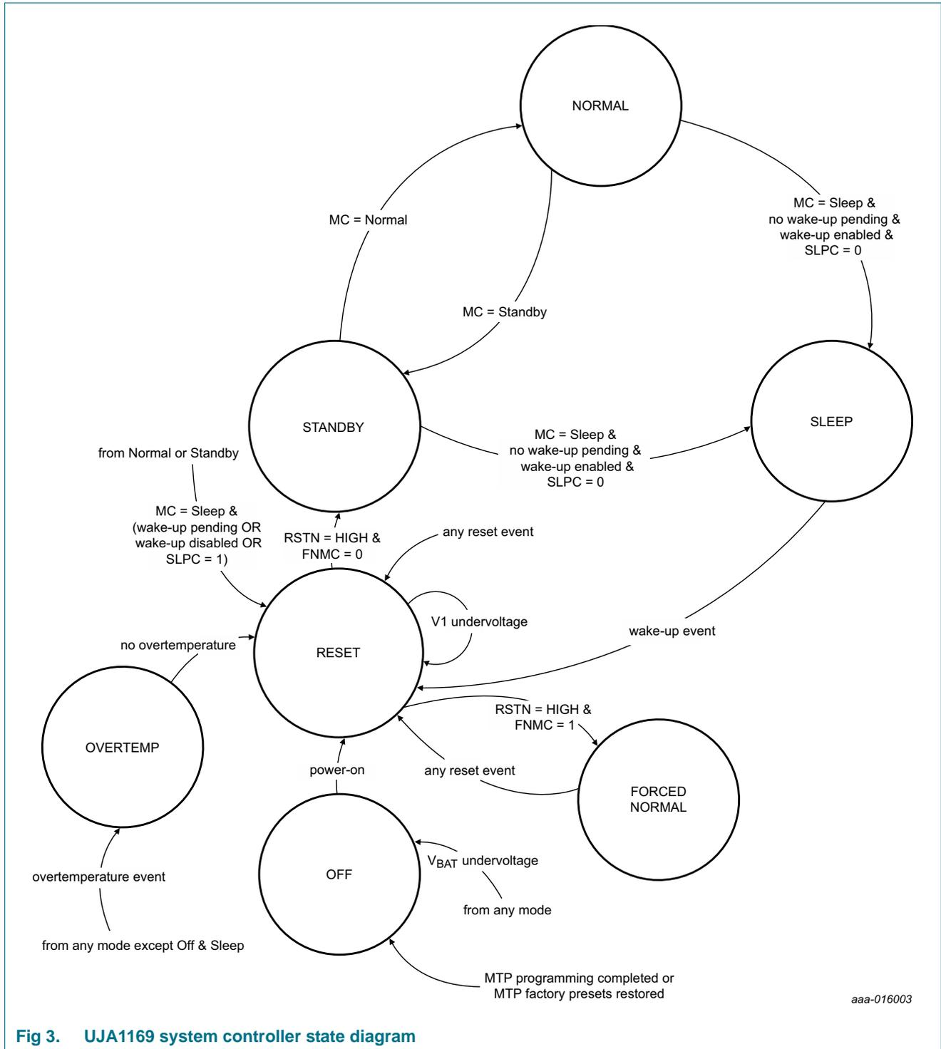
Fig 3. UJA1169 system controller state diagram
