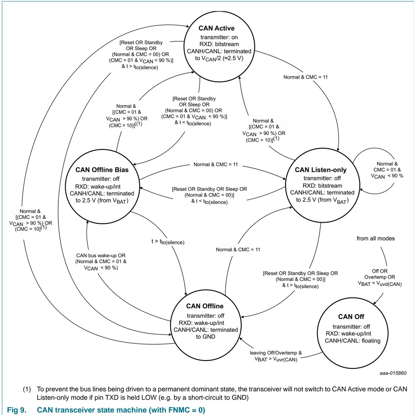
Fig 9. CAN transceiver state machine (with FNMC = 0)
