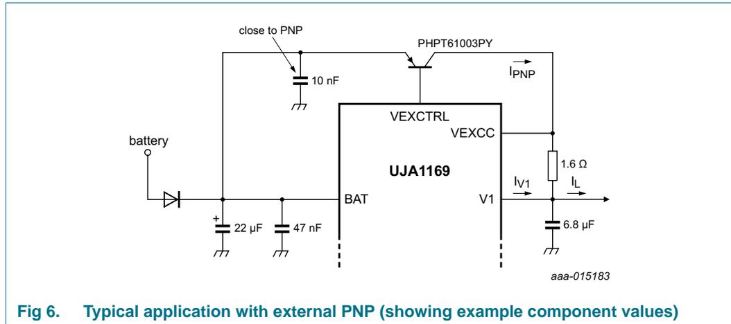
**Fig 6. Typical application with external PNP (showing example component values)**
