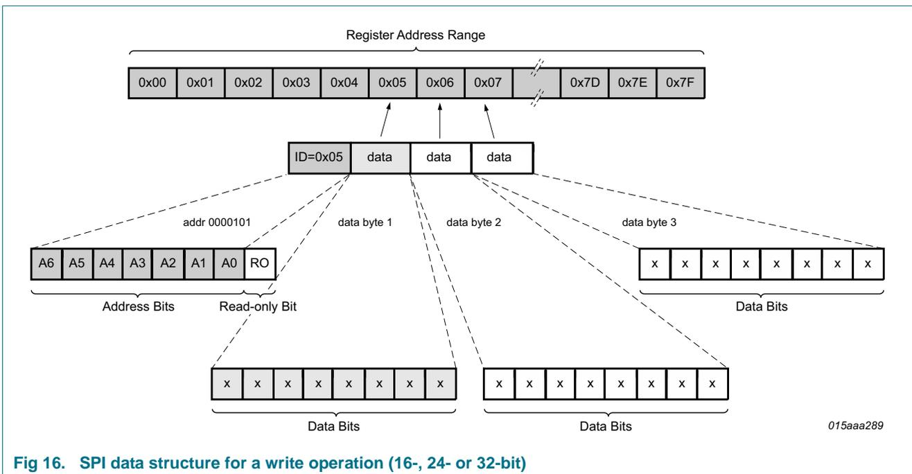
Fig 16. SPI data structure for a write operation (16-, 24- or 32-bit)
