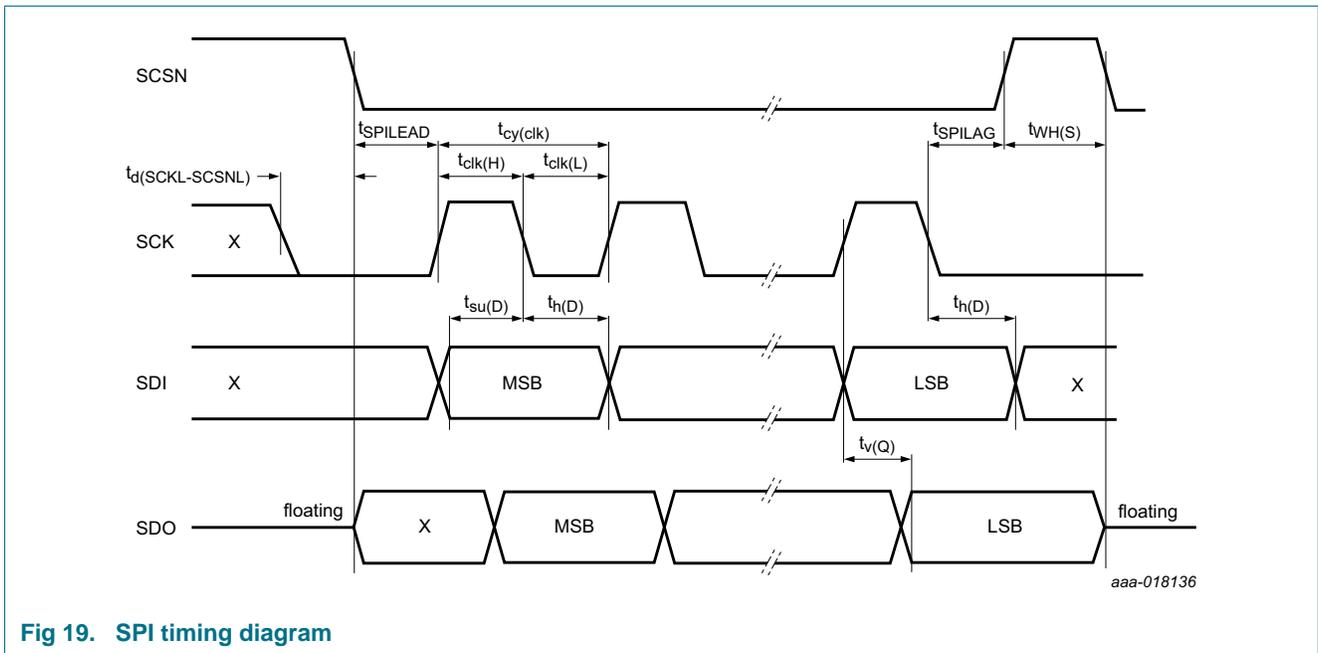
Fig 19. SPI timing diagram
