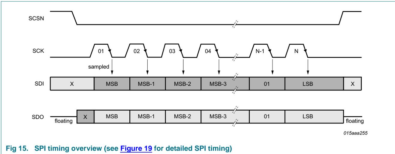
Fig 15. SPI timing overview (see [Figure 19](#) for detailed SPI timing)
