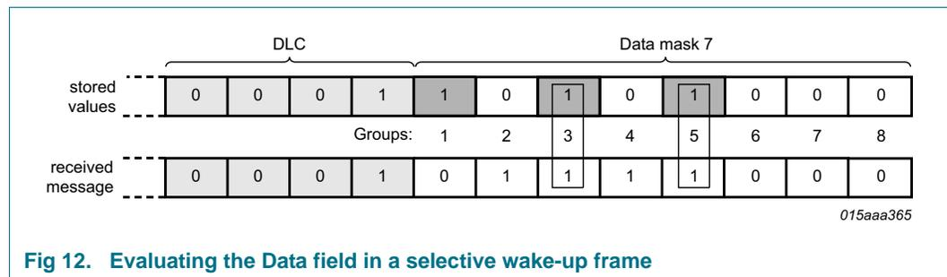
**Fig 12. Evaluating the Data field in a selective wake-up frame**
