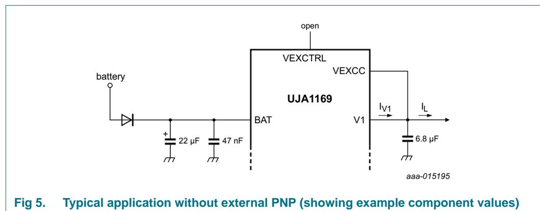
**Fig 5. Typical application without external PNP (showing example component values)**
