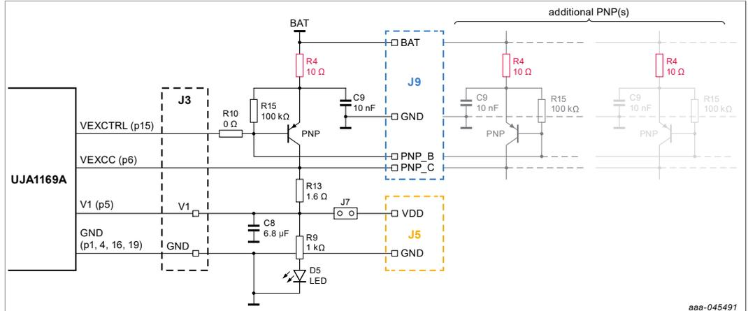
Figure 7. Simplified schematic of UJA1169Ax-EVB with multiple PNPs.
