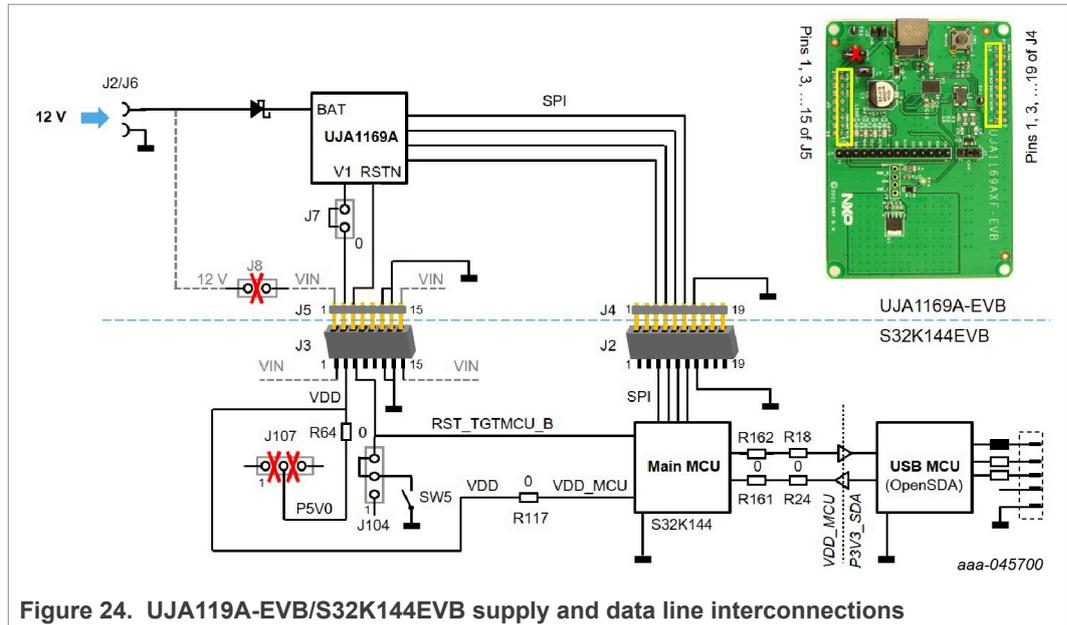
Figure 24. UJA119A-EVB/S32K144EVB supply and data line interconnections
