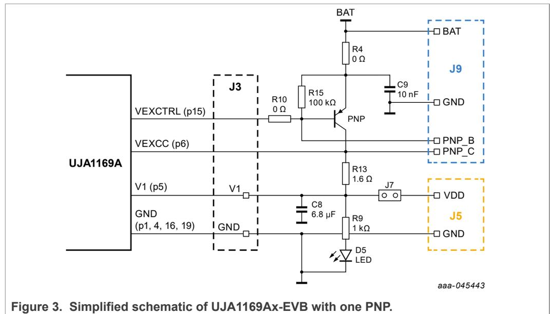
Figure 3. Simplified schematic of UJA1169Ax-EVB with one PNP.
