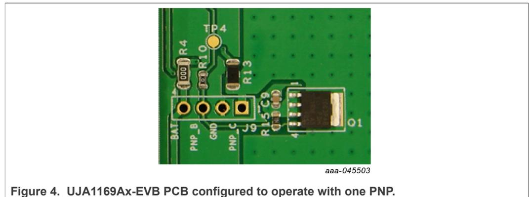
Figure 4. UJA1169Ax-EVB PCB configured to operate with one PNP.
