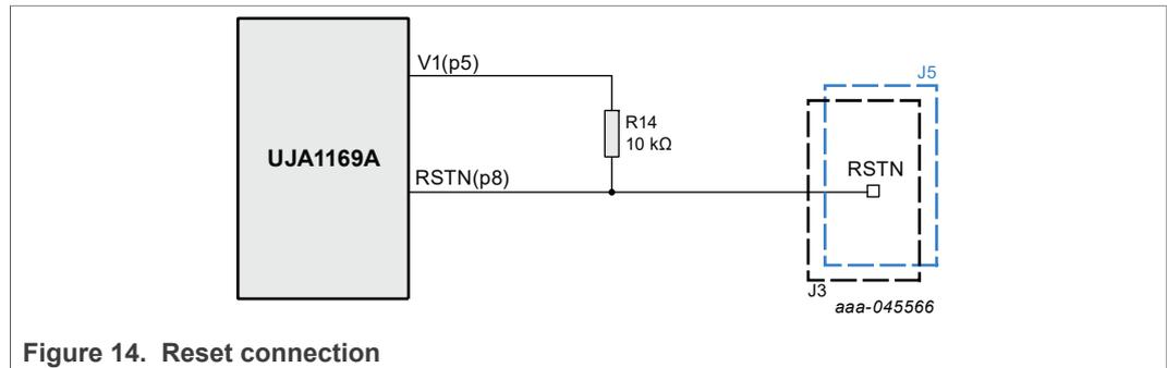
Figure 14. Reset connection
