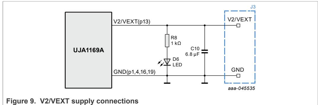
Figure 9. V2/VEXT supply connections
