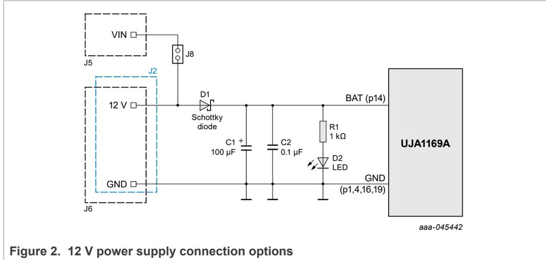
Figure 2. 12 V power supply connection options
