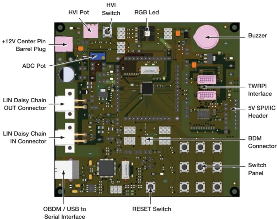
Figure 1: Front side of TRK-S12ZVL
