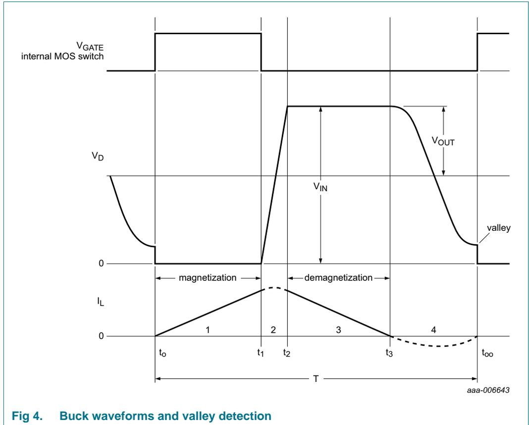
Fig 4. Buck waveforms and valley detection
