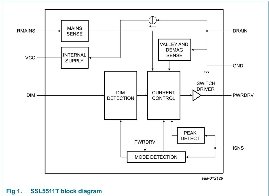
Fig 1. SSL5511T block diagram
