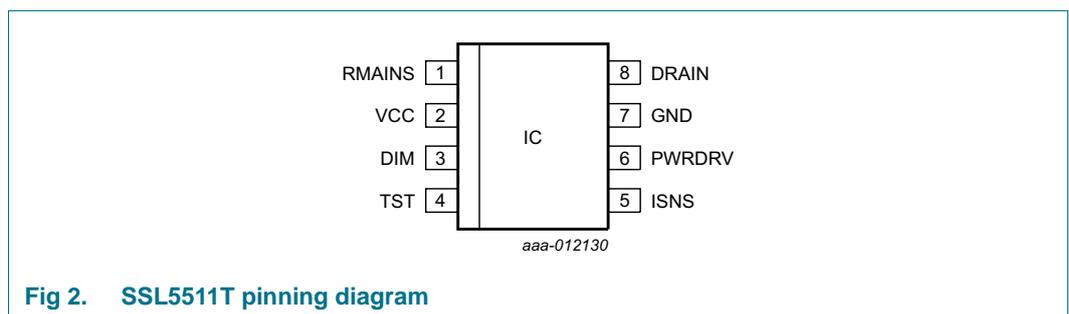
Fig 2. SSL5511T pinning diagram
