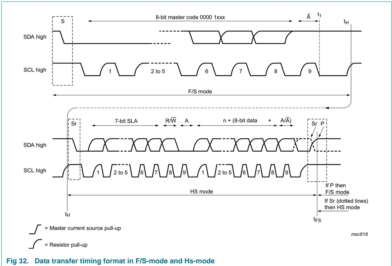
Fig 32. Data transfer timing format in F/S-mode and HS-mode
