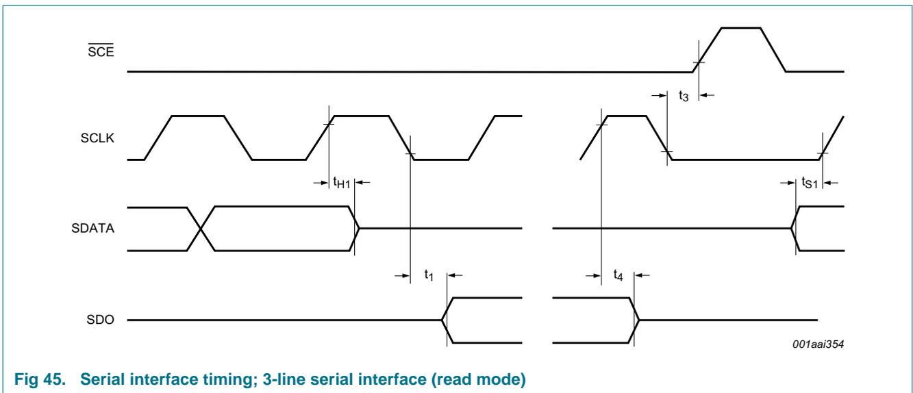
Fig 45. Serial interface timing; 3-line serial interface (read mode)
