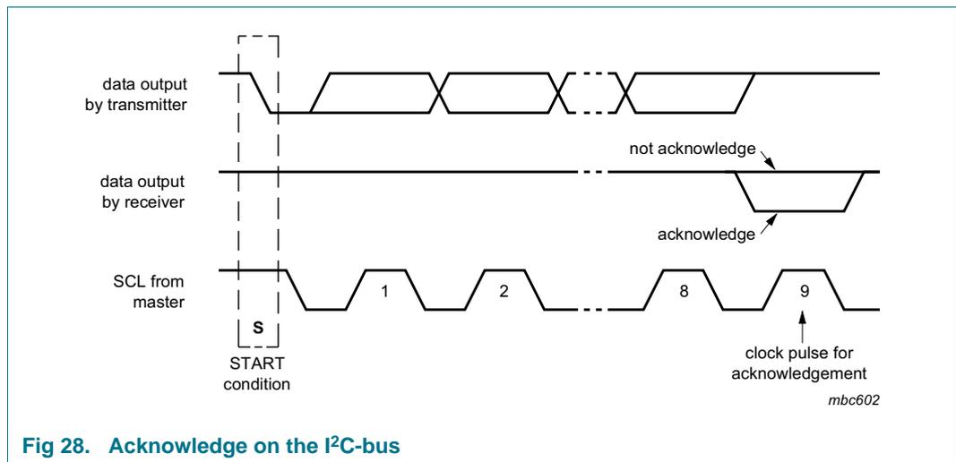
Fig 28. Acknowledge on the I<sup>2</sup>C-bus
