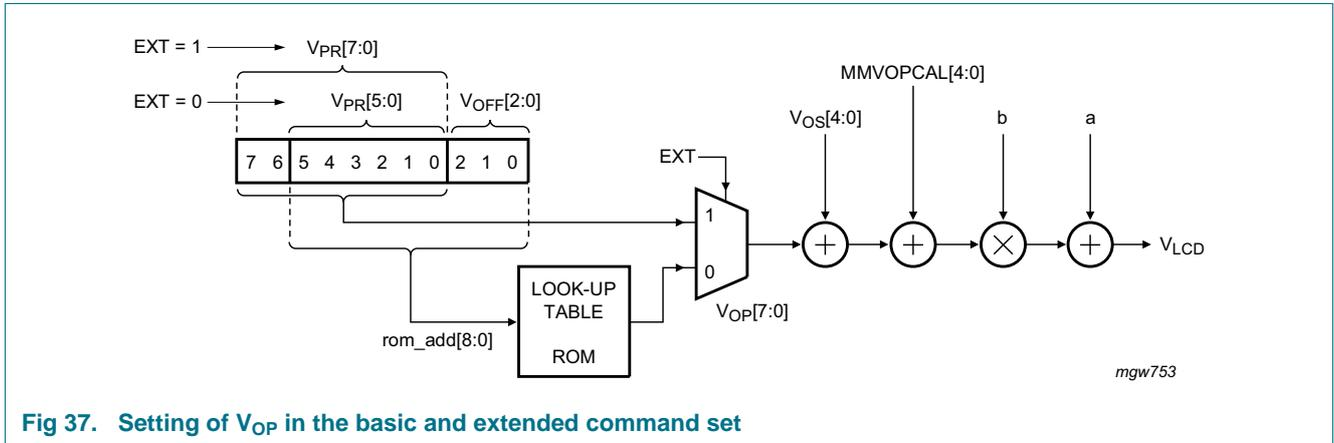
Fig 37. Setting of  $V_{OP}$  in the basic and extended command set
