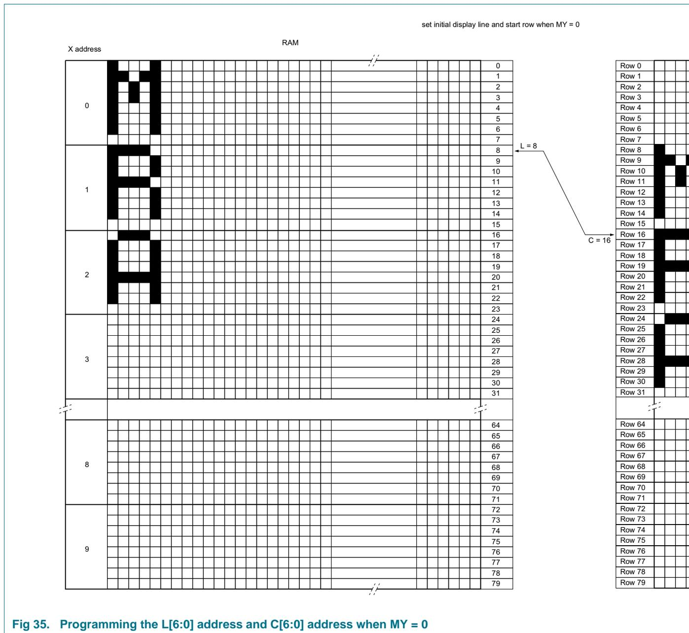
Fig 35. Programming the L[6:0] address and C[6:0] address when MY = 0
