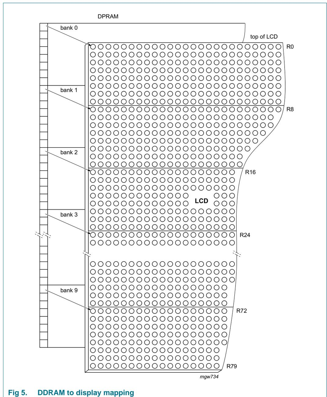
Fig 5. DDRAM to display mapping
