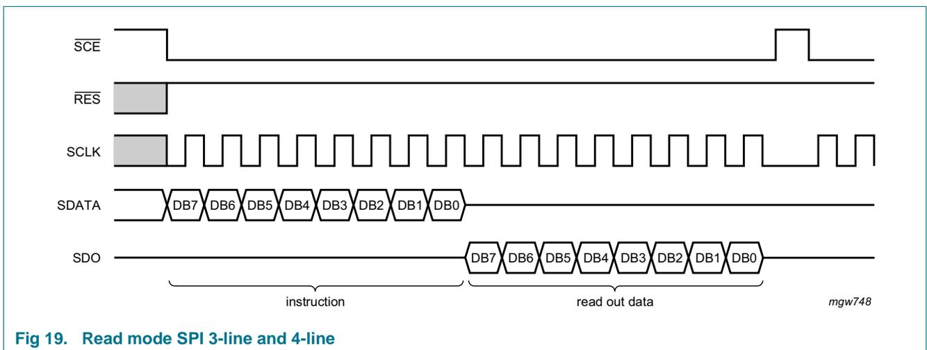
Fig 19. Read mode SPI 3-line and 4-line
