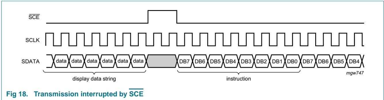
Fig 18. Transmission interrupted by  $\overline{SCE}$
