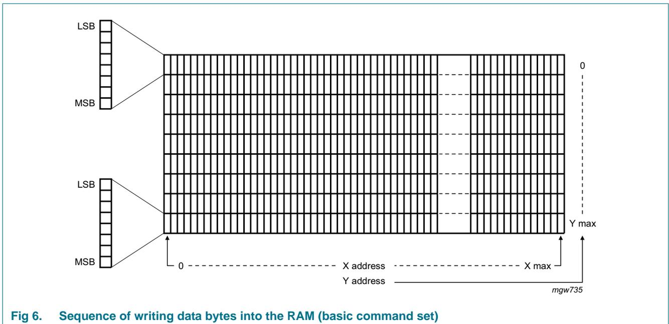
Fig 6. Sequence of writing data bytes into the RAM (basic command set)
