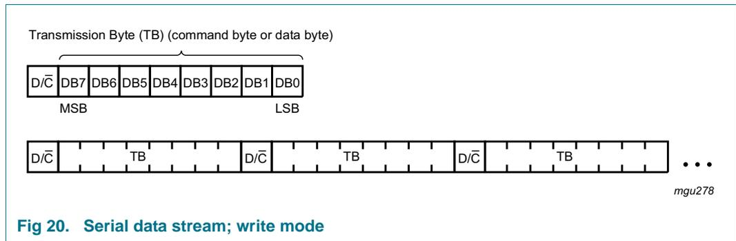
**Fig 20. Serial data stream; write mode**
