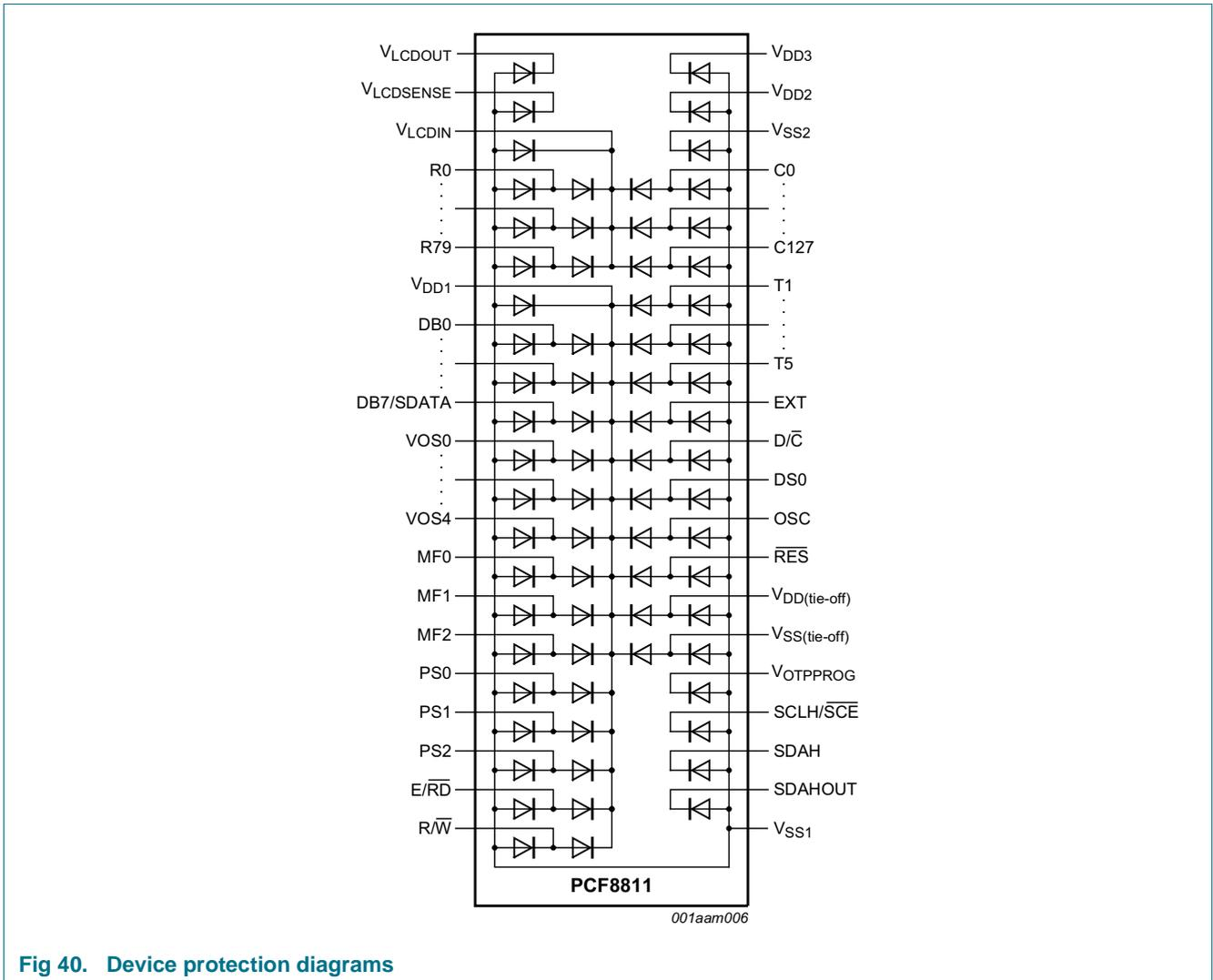
Fig 40. Device protection diagrams
