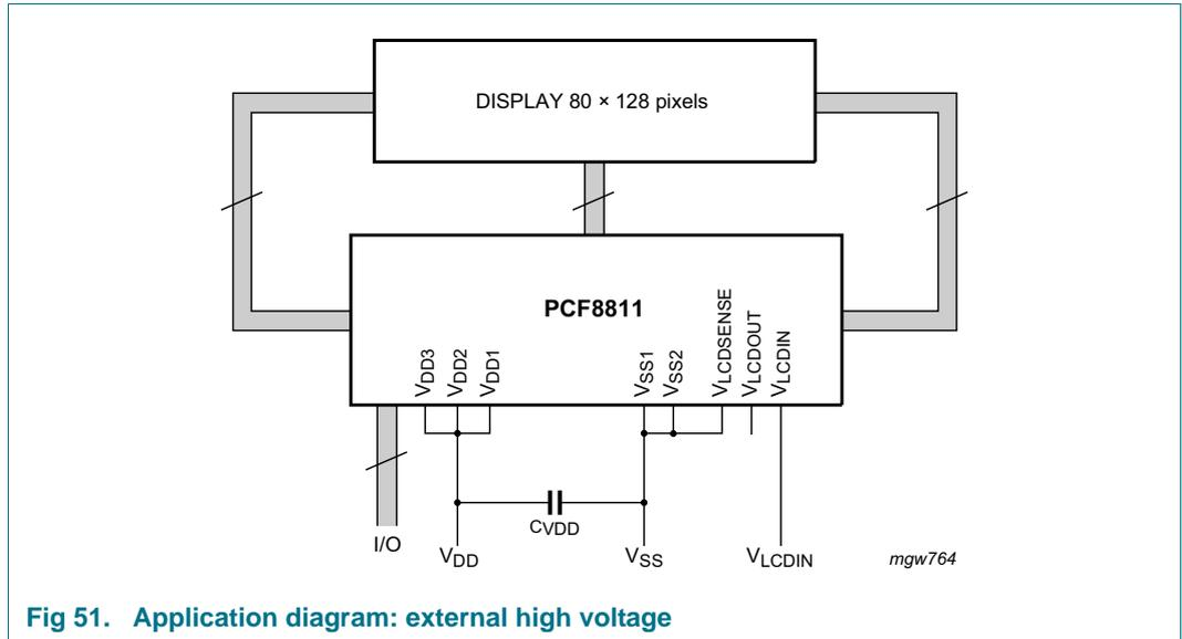
Fig 51. Application diagram: external high voltage
