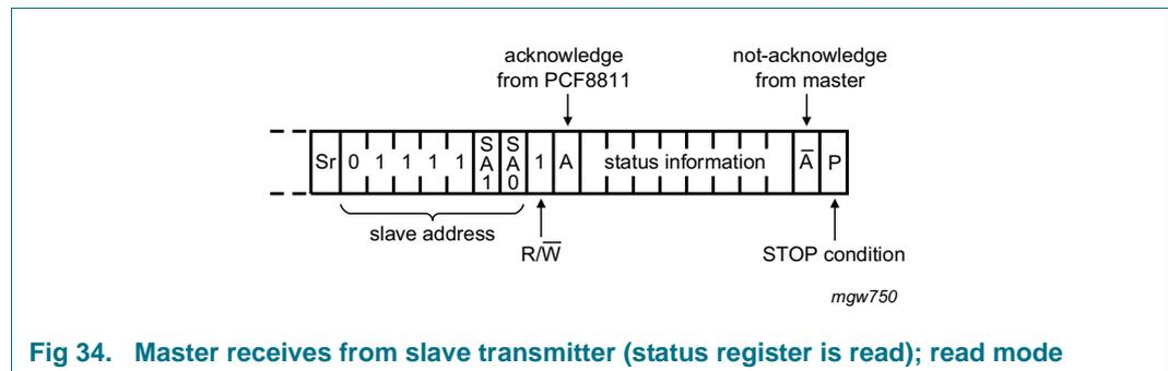
Fig 34. Master receives from slave transmitter (status register is read); read mode
