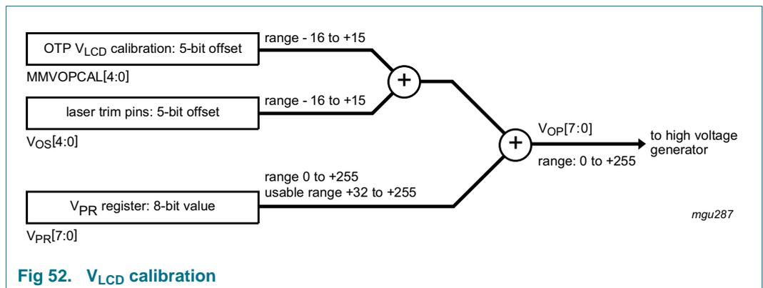
Fig 52.  $V_{LCD}$  calibration
