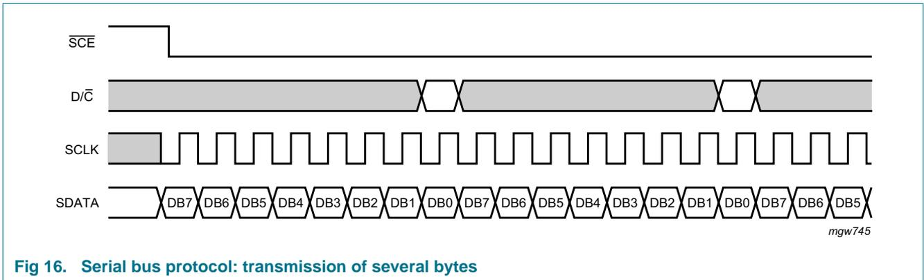
Fig 16. Serial bus protocol: transmission of several bytes
