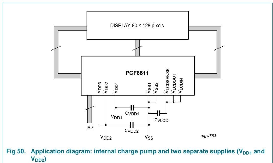
Fig 50. Application diagram: internal charge pump and two separate supplies ( $V_{DD1}$  and  $V_{DD2}$ )
