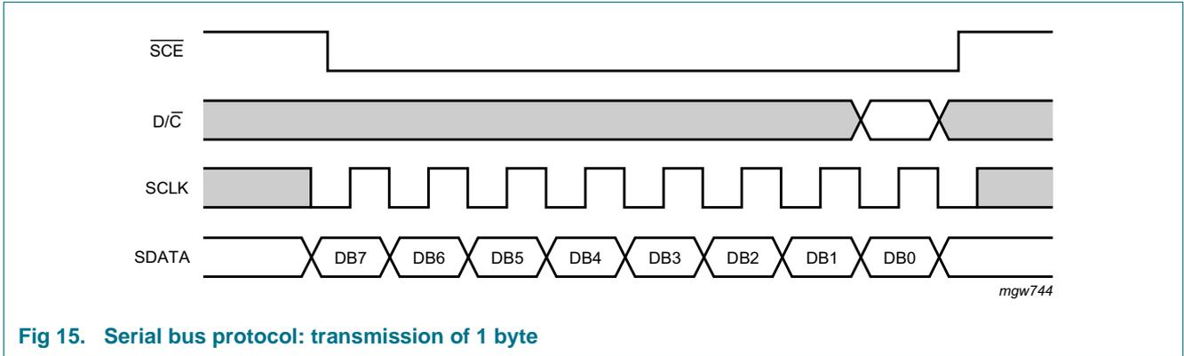
Fig 15. Serial bus protocol: transmission of 1 byte
