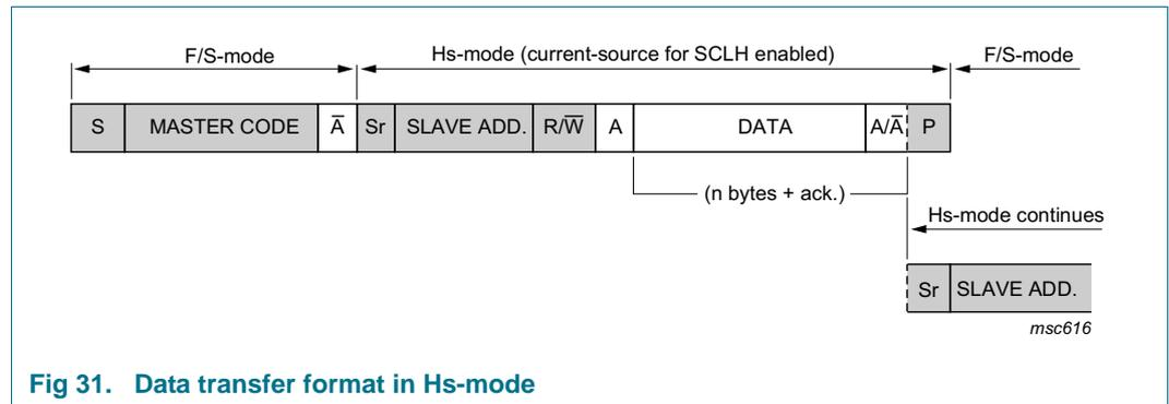
Fig 31. Data transfer format in Hs-mode
