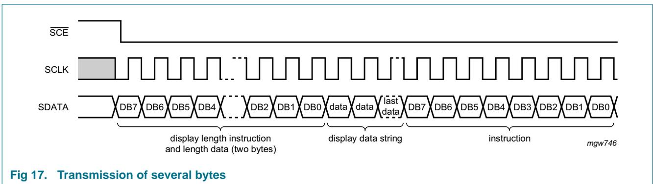
Fig 17. Transmission of several bytes
