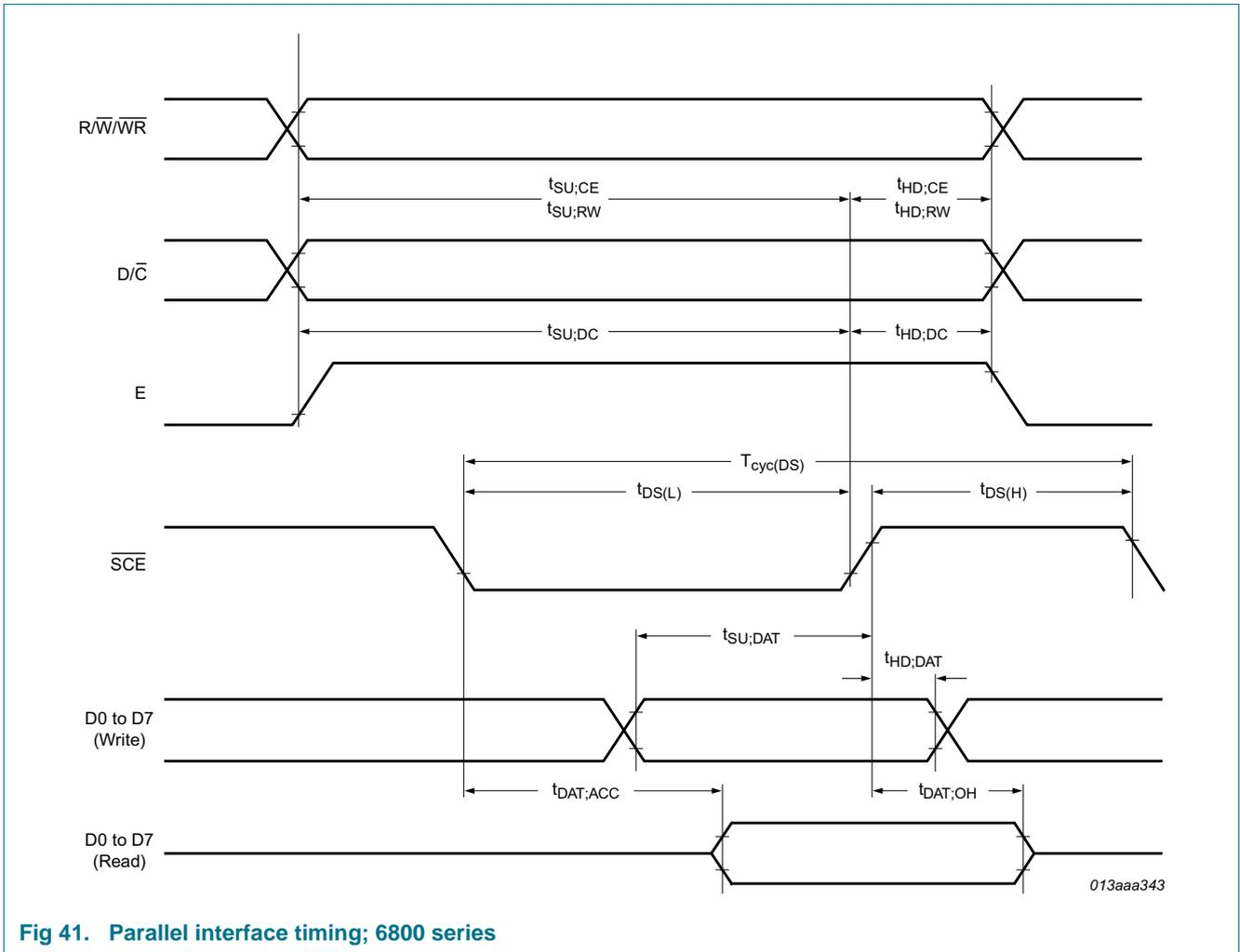
Fig 41. Parallel interface timing; 6800 series
