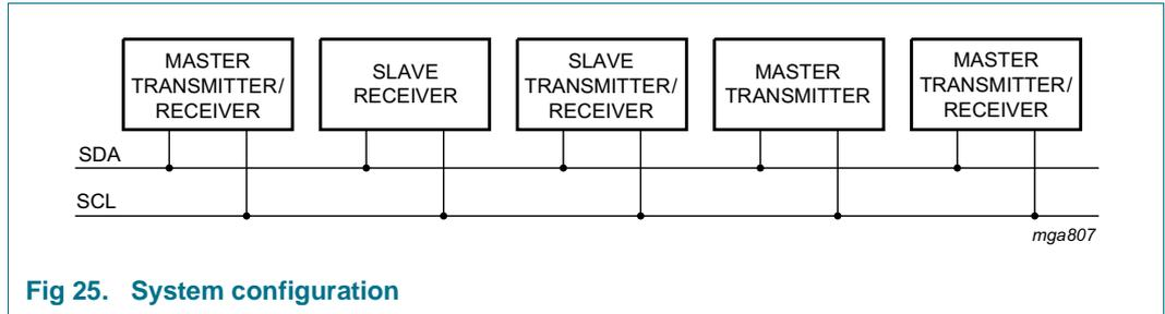
Fig 25. System configuration
