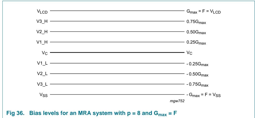
**Fig 36. Bias levels for an MRA system with  $p = 8$  and  $G_{max} = F$**
