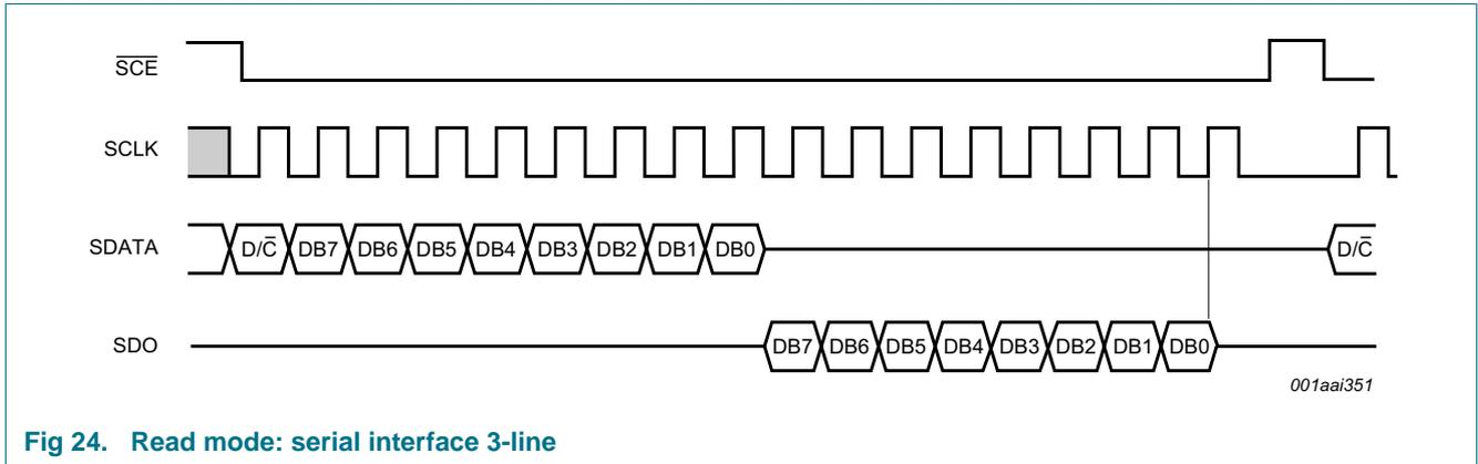
Fig 24. Read mode: serial interface 3-line
