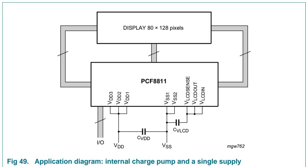
Fig 49. Application diagram: internal charge pump and a single supply
