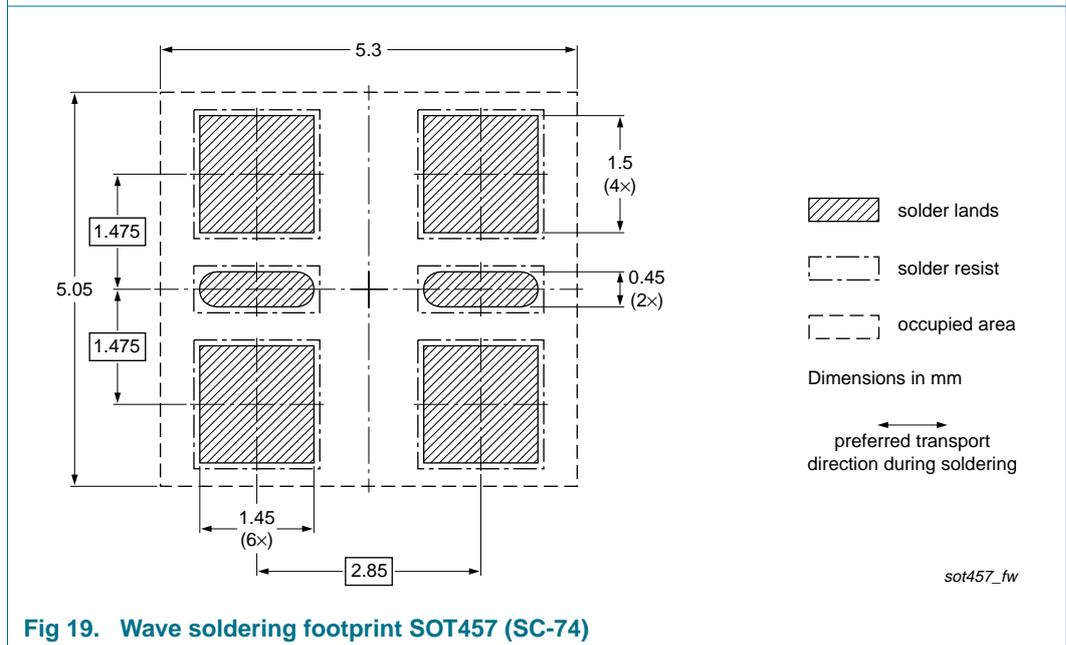
**Fig 19. Wave soldering footprint SOT457 (SC-74)**
