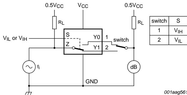
Adjust  $f_i$  voltage to obtain 0 dBm level at input.
