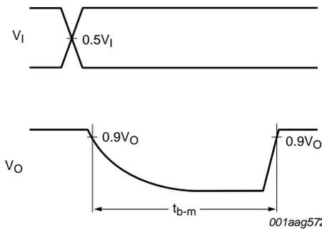
b. Input and output measurement points
