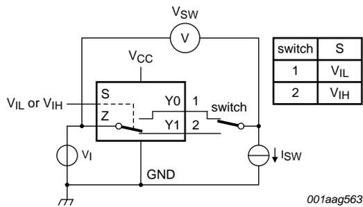
$R_{ON} = V_{SW} / I_{sw}$ .
