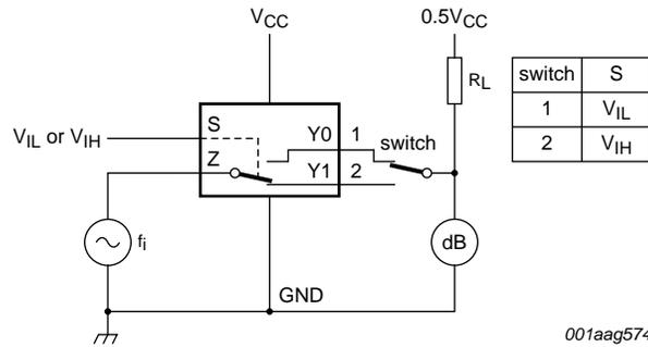
Adjust  $f_i$  voltage to obtain 0 dBm level at output. Increase  $f_i$  frequency until dB meter reads -3 dB.
