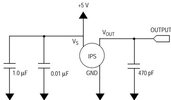
Figure 4. Recommended power supply decoupling and output filtering
