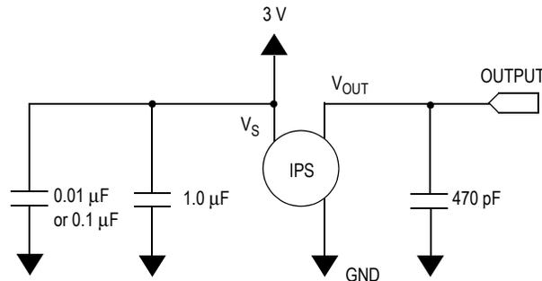
Figure 5. Recommended power supply decoupling and output filtering
