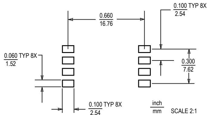
**Figure 9. SOP footprint (case 98ASB17757C)**
