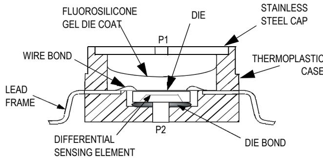
Figure 4. Cross-sectional diagram SOP (not to scale)
