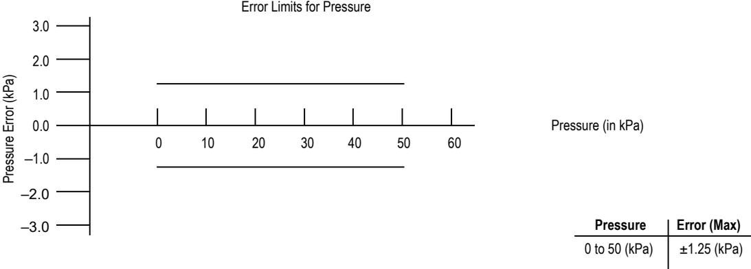
**Figure 8. Pressure error band**
