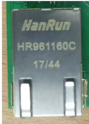
Figure 6. Ethernet connector RJ45
