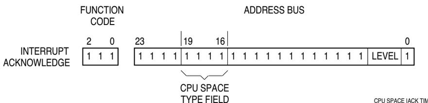
**Figure 4-19 CPU Space Encoding for Interrupt Acknowledge**
