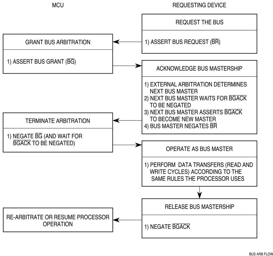
**Figure 4-14 Bus Arbitration Flowchart for Single Request**
