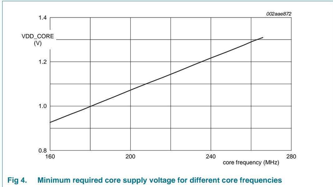
Fig 4. Minimum required core supply voltage for different core frequencies
