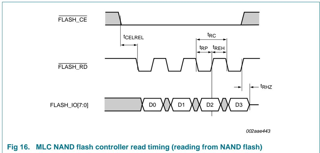
Fig 16. MLC NAND flash controller read timing (reading from NAND flash)
