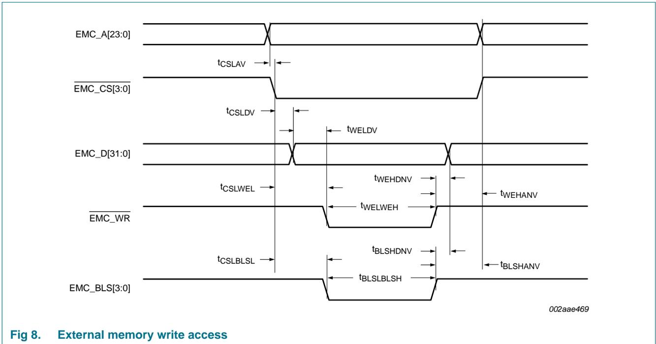
Fig 8. External memory write access
