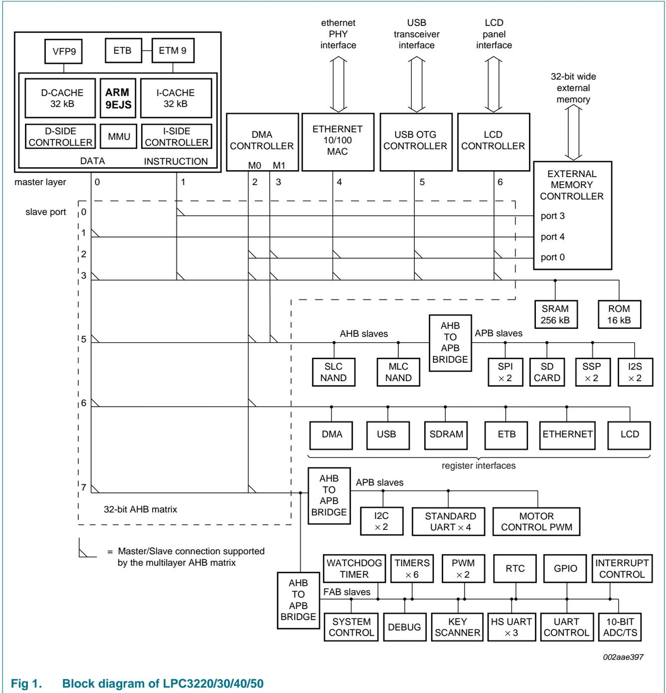
Fig 1. Block diagram of LPC3220/30/40/50
