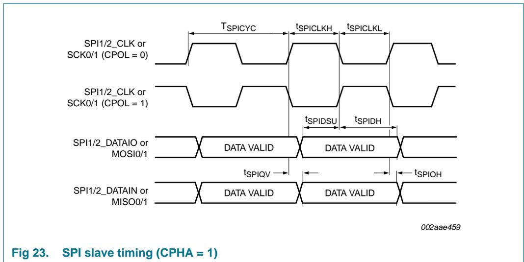
Fig 23. SPI slave timing (CPHA = 1)
