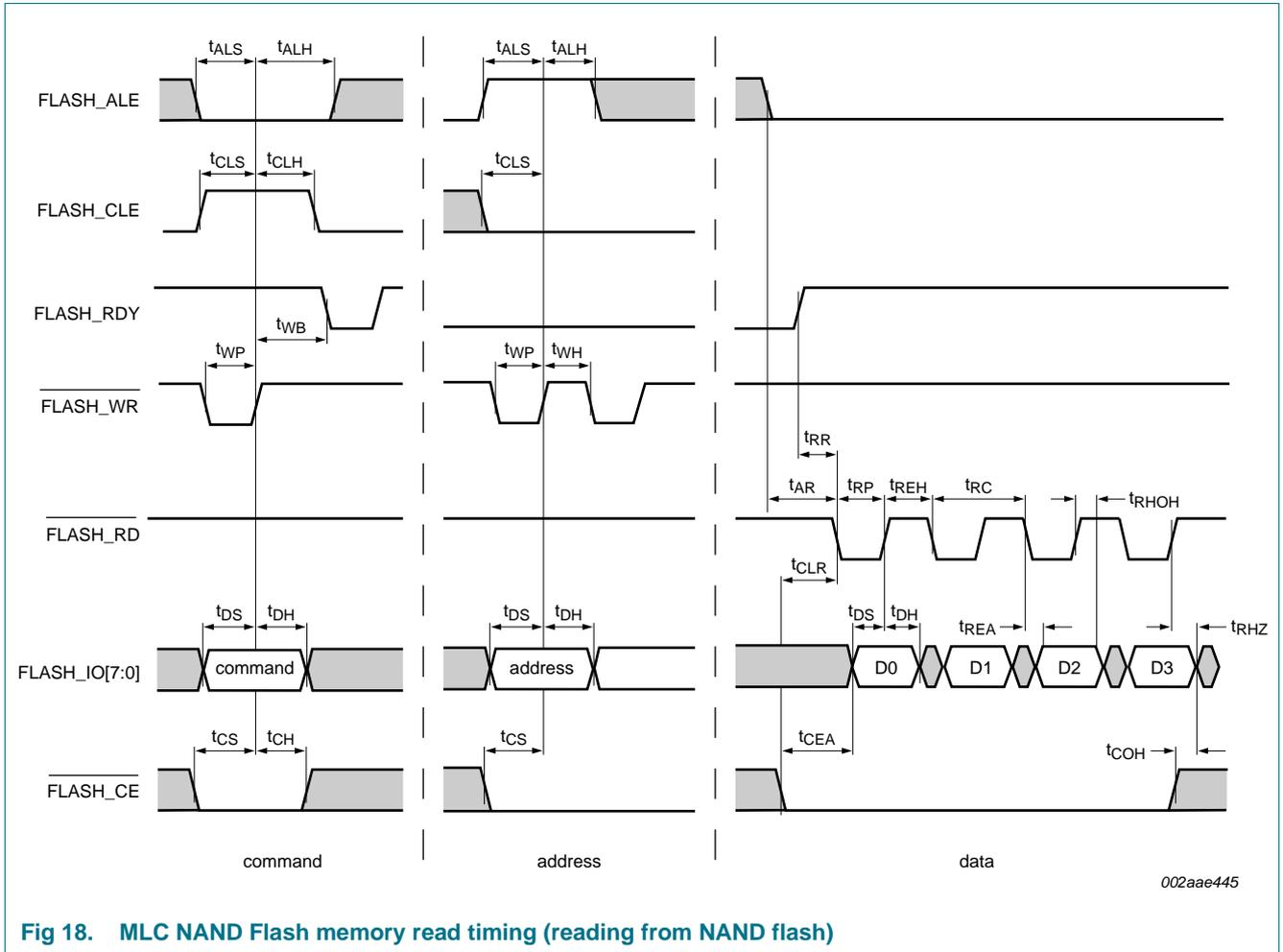
Fig 18. MLC NAND Flash memory read timing (reading from NAND flash)
