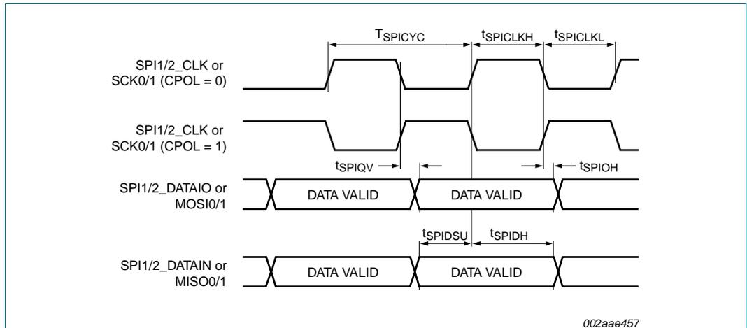
Fig 20. SPI master timing (CPHA = 0)
