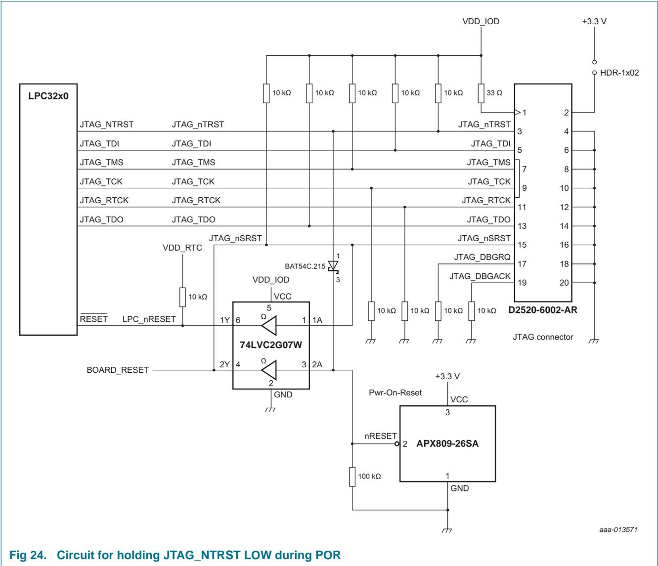
Fig 24. Circuit for holding JTAG\_NTRST LOW during POR
