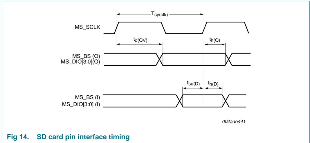
Fig 14. SD card pin interface timing
