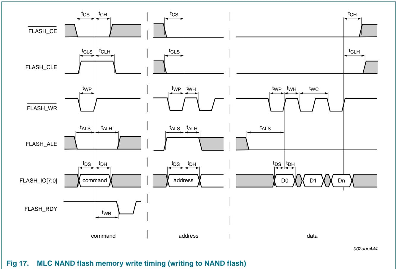
Fig 17. MLC NAND flash memory write timing (writing to NAND flash)
