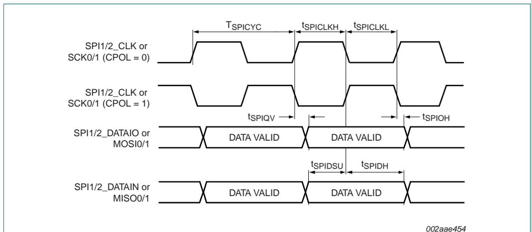
Fig 21. SPI master timing (CPHA = 1)
