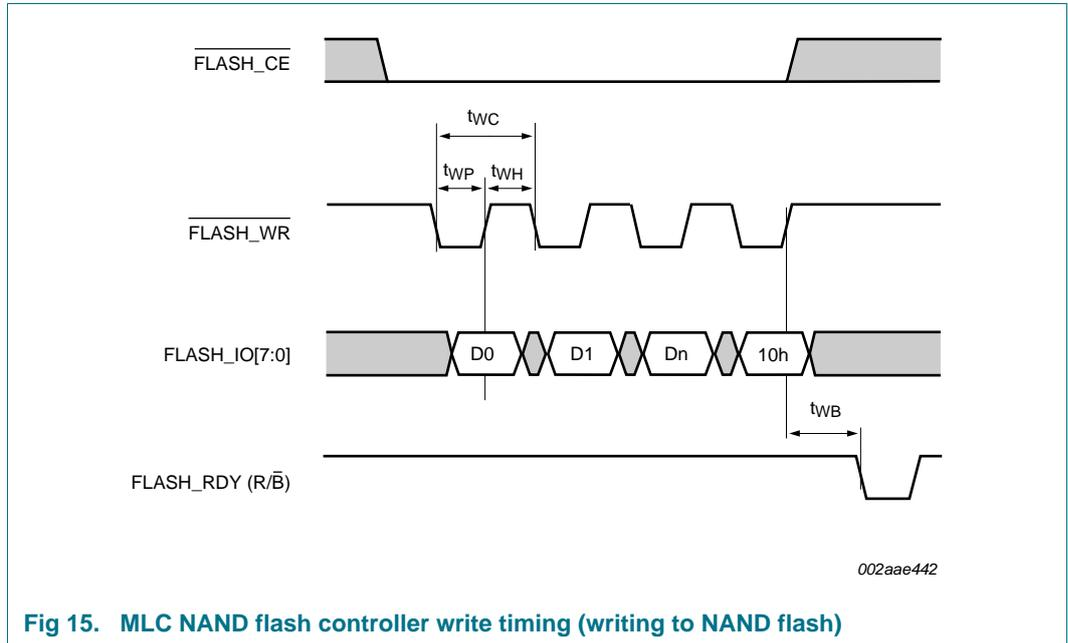
Fig 15. MLC NAND flash controller write timing (writing to NAND flash)
