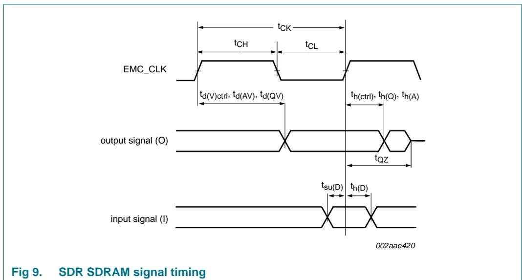
**Fig 9. SDR SDRAM signal timing**
