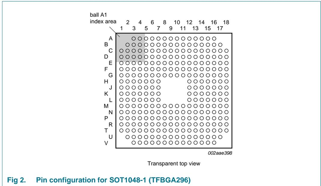
Fig 2. Pin configuration for SOT1048-1 (TFBGA296)
