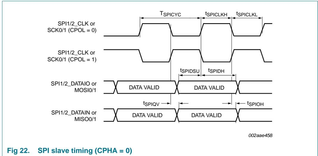
Fig 22. SPI slave timing (CPHA = 0)
