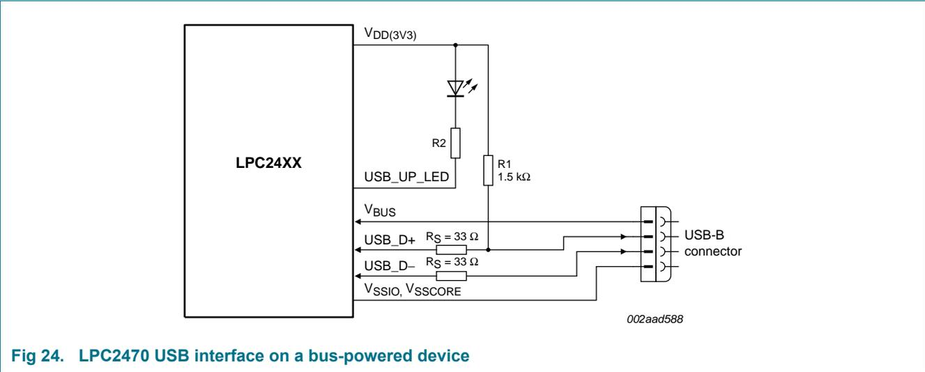
Fig 24. LPC2470 USB interface on a bus-powered device
