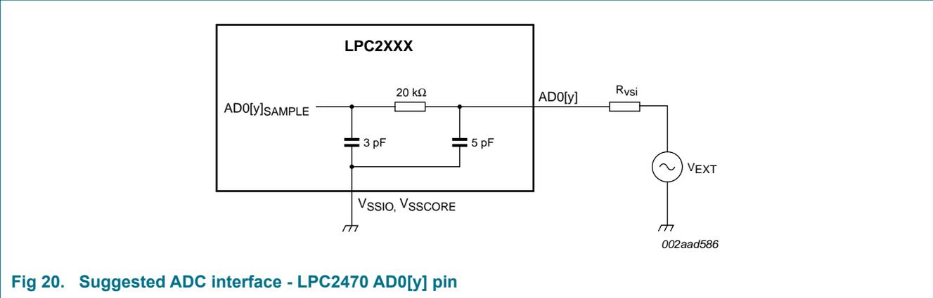
Fig 20. Suggested ADC interface - LPC2470 AD0[y] pin
