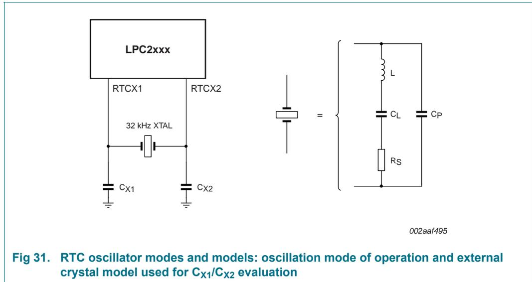
The RTC external oscillator circuit is shown in [Figure 31](#). Since the feedback resistance is integrated on chip, only a crystal, the capacitances  $C_{X1}$  and  $C_{X2}$  need to be connected externally to the microcontroller.
