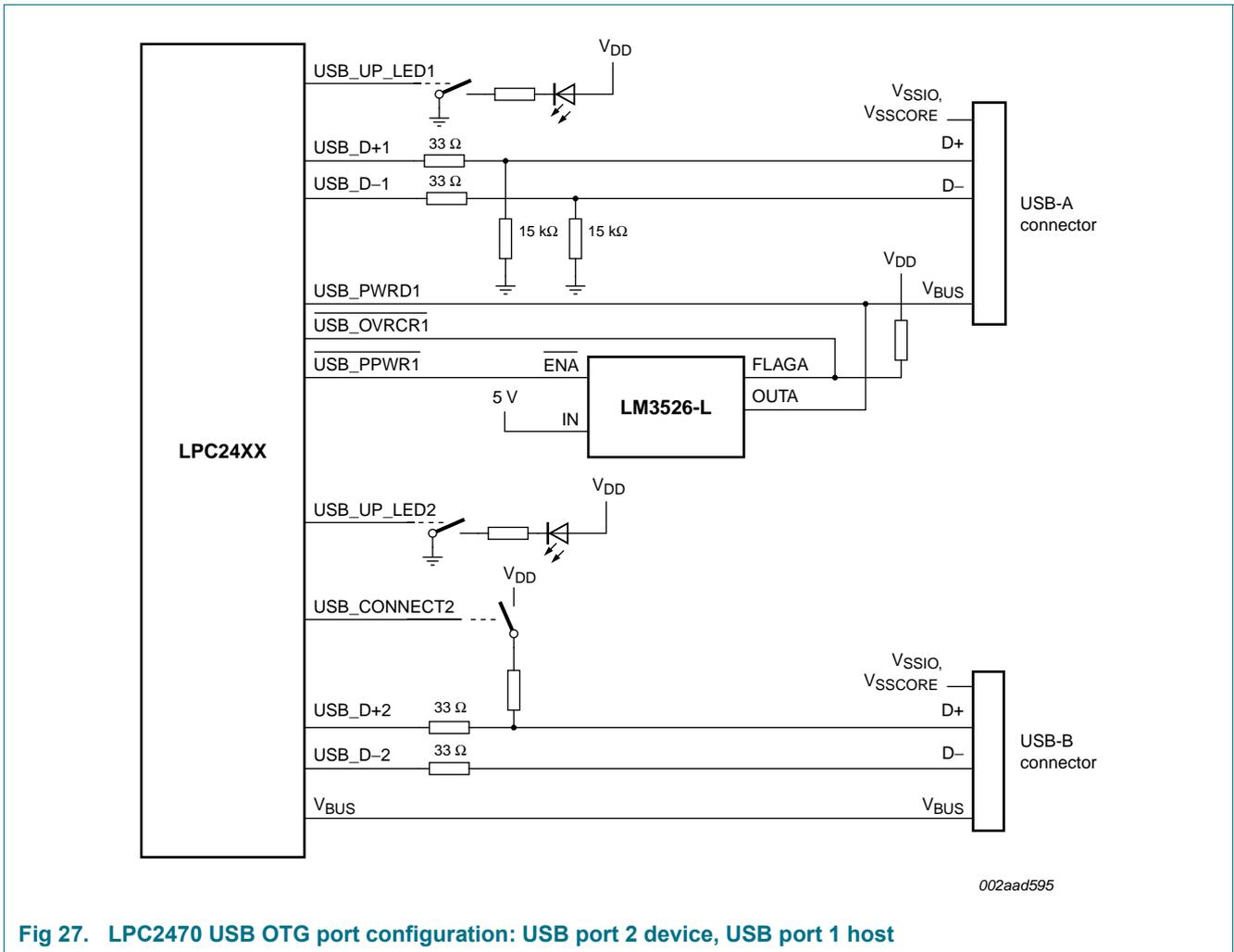
Fig 27. LPC2470 USB OTG port configuration: USB port 2 device, USB port 1 host
