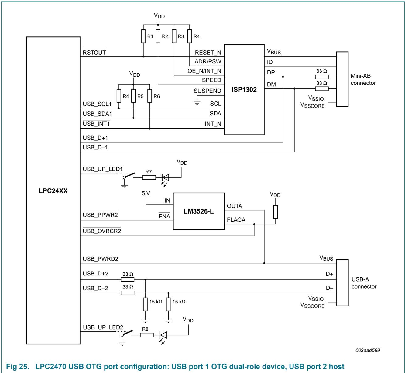
Fig 25. LPC2470 USB OTG port configuration: USB port 1 OTG dual-role device, USB port 2 host
