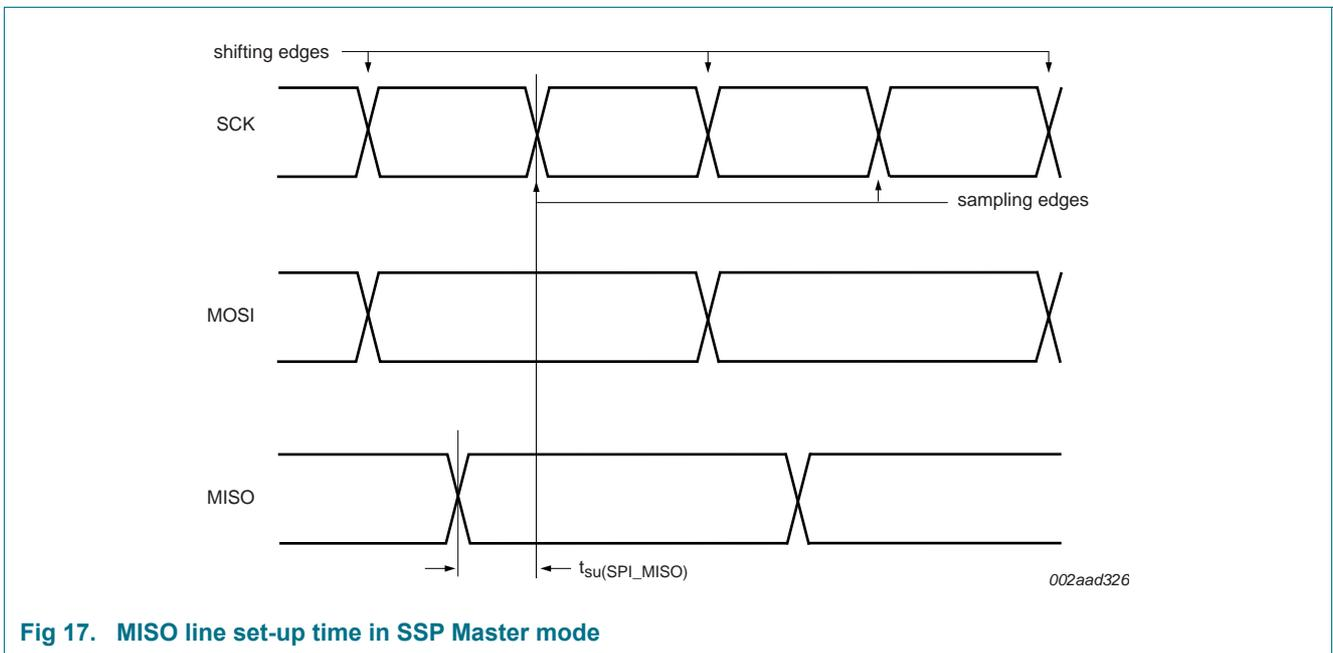
Fig 17. MISO line set-up time in SSP Master mode
