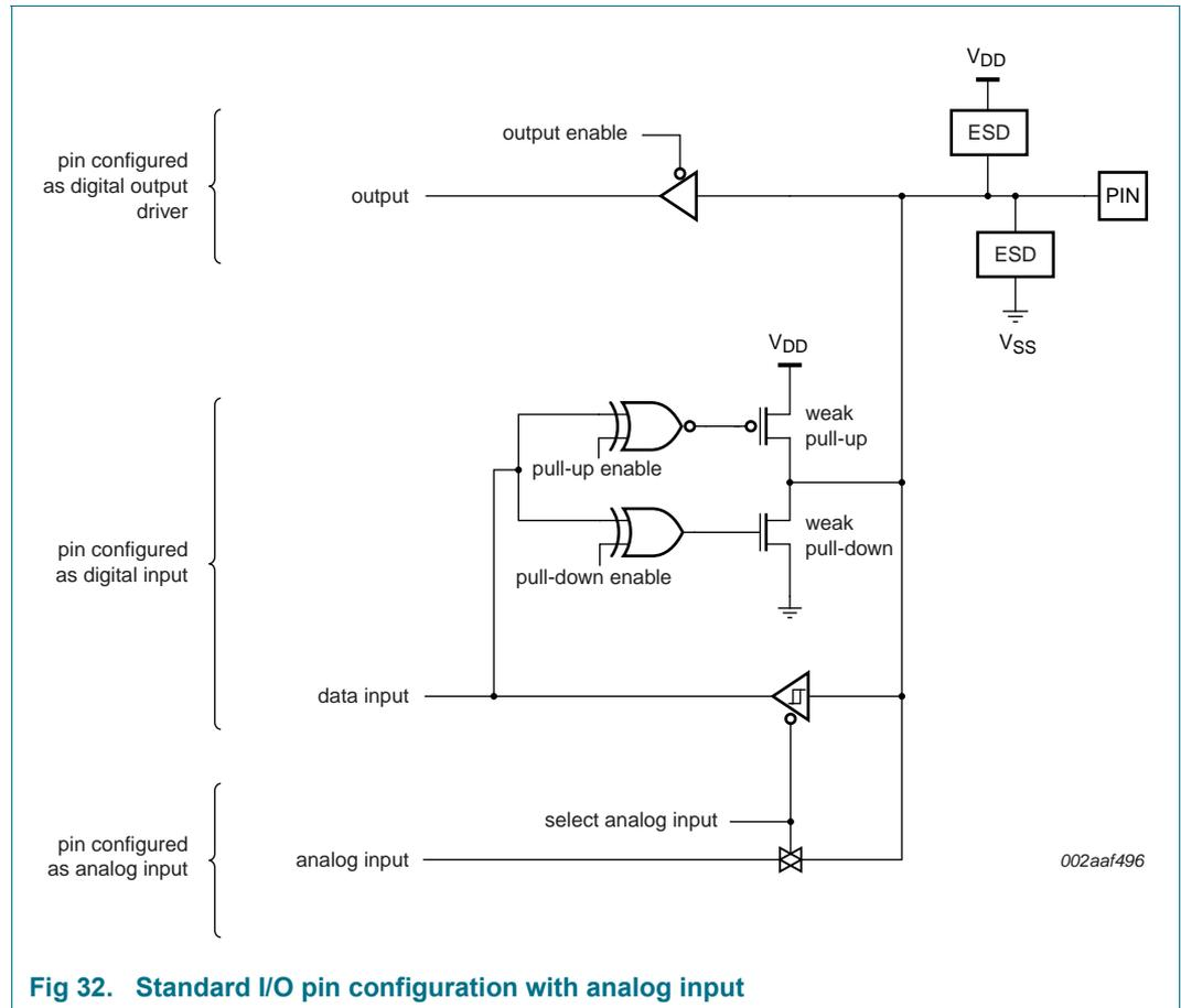
Fig 32. Standard I/O pin configuration with analog input
