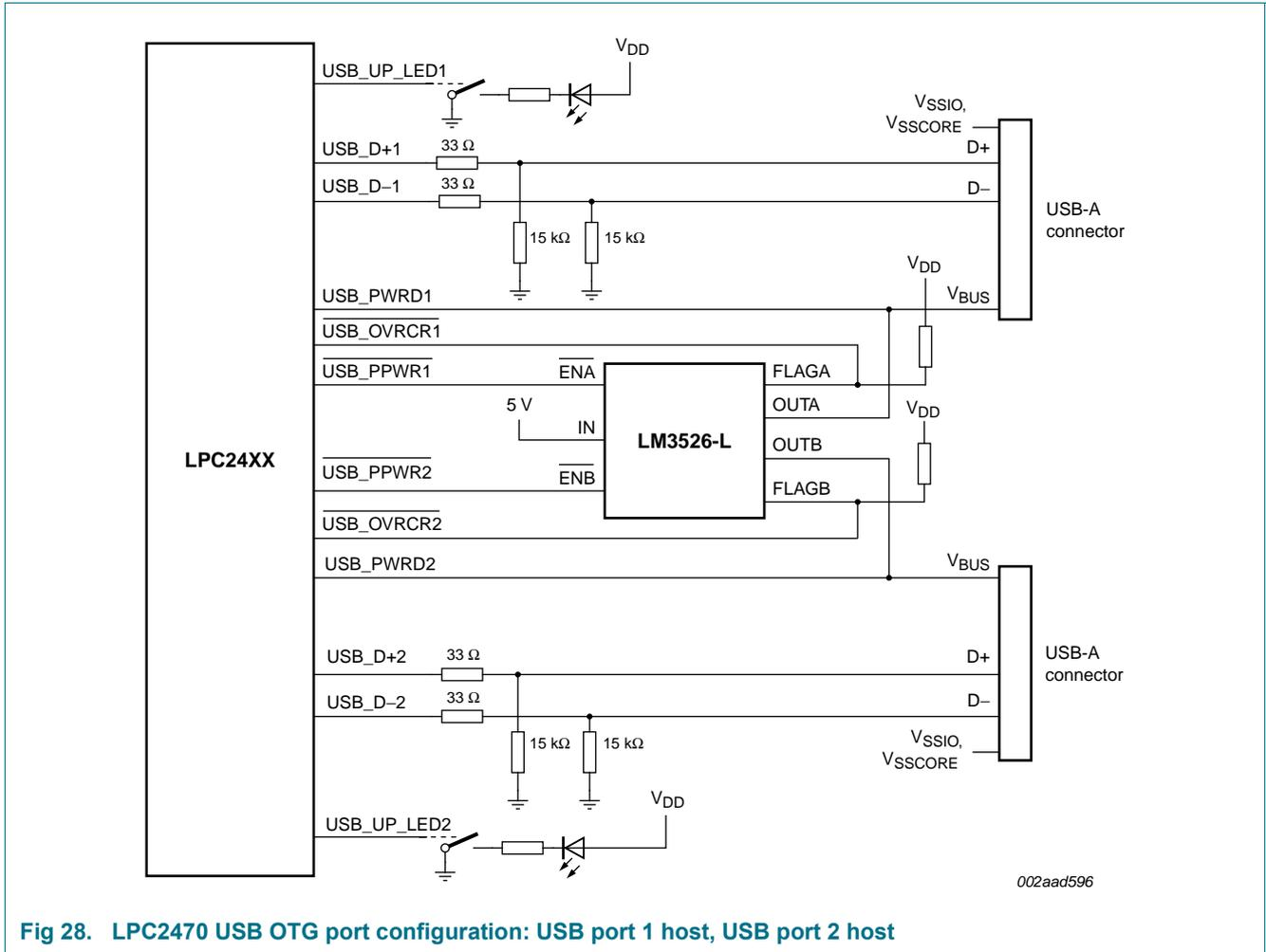
Fig 28. LPC2470 USB OTG port configuration: USB port 1 host, USB port 2 host
