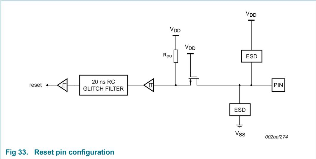
Fig 33. Reset pin configuration
