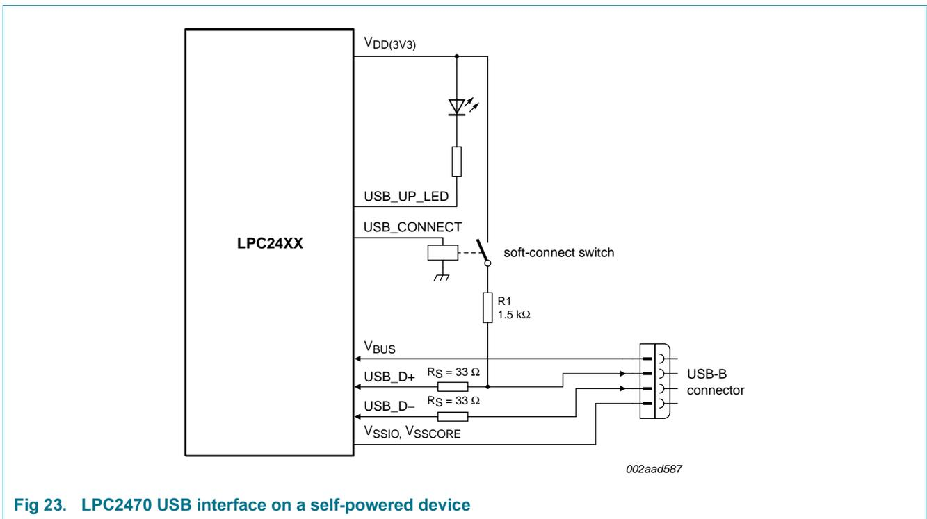
Fig 23. LPC2470 USB interface on a self-powered device
