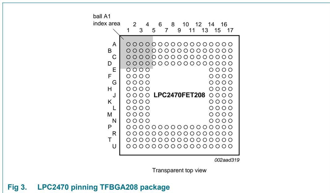
Fig 3. LPC2470 pinning TFBGA208 package
