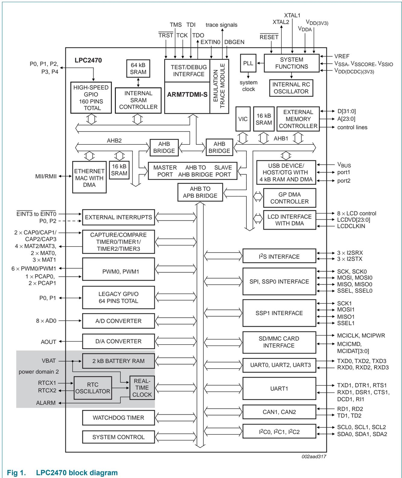
Fig 1. LPC2470 block diagram
