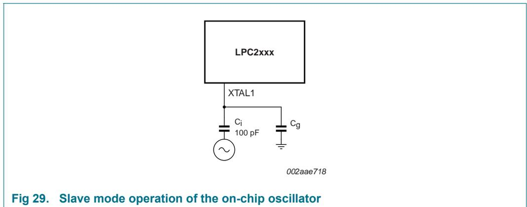
Fig 29. Slave mode operation of the on-chip oscillator
