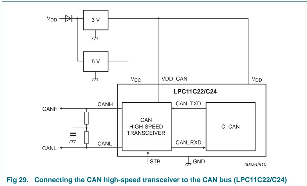
Fig 29. Connecting the CAN high-speed transceiver to the CAN bus (LPC11C22/C24)
