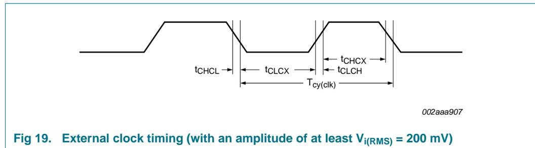
**Fig 19. External clock timing (with an amplitude of at least  $V_{i(RMS)} = 200\text{ mV}$ )**
