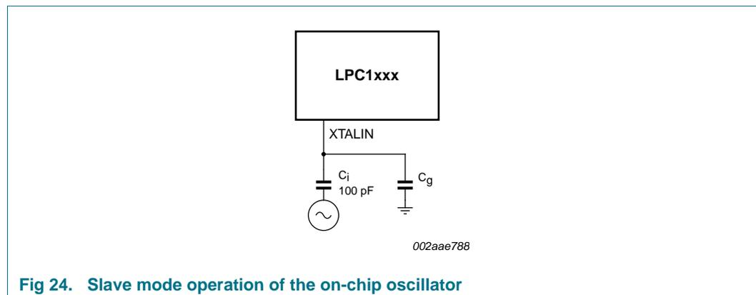
**Fig 24. Slave mode operation of the on-chip oscillator**
