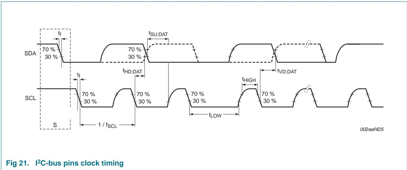
Fig 21. I<sup>2</sup>C-bus pins clock timing
