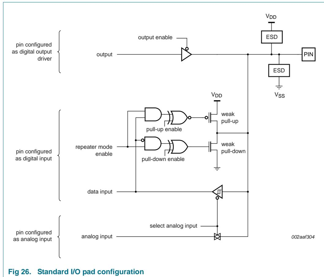
Fig 26. Standard I/O pad configuration
