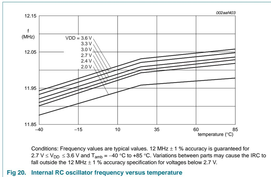
**Fig 20. Internal RC oscillator frequency versus temperature**
