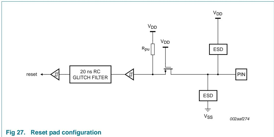
Fig 27. Reset pad configuration
