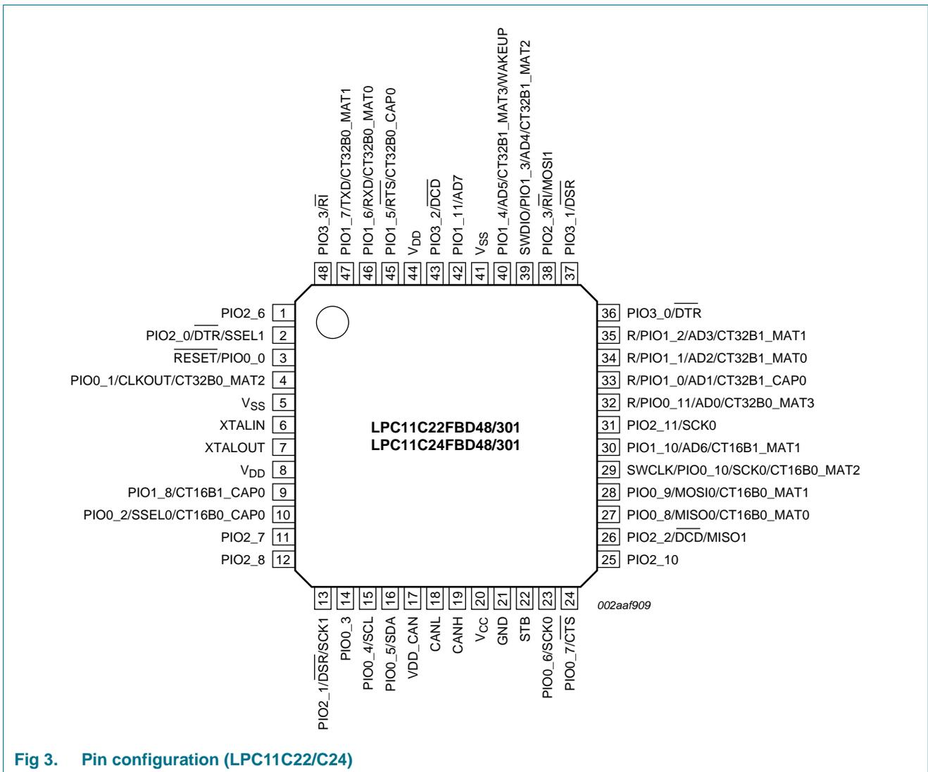
Fig 3. Pin configuration (LPC11C22/C24)
