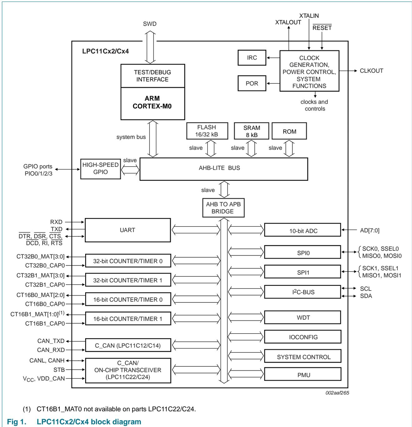
Fig 1. LPC11Cx2/Cx4 block diagram
