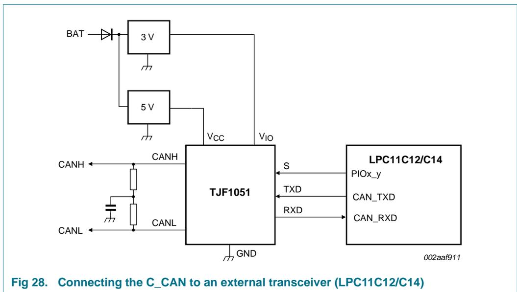
Fig 28. Connecting the C\_CAN to an external transceiver (LPC11C12/C14)
