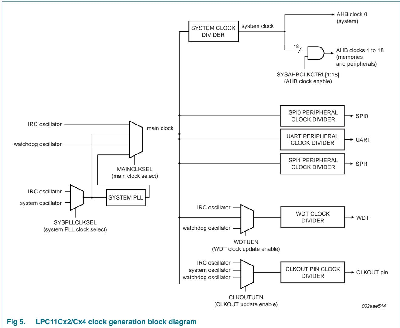
Fig 5. LPC11Cx2/Cx4 clock generation block diagram
