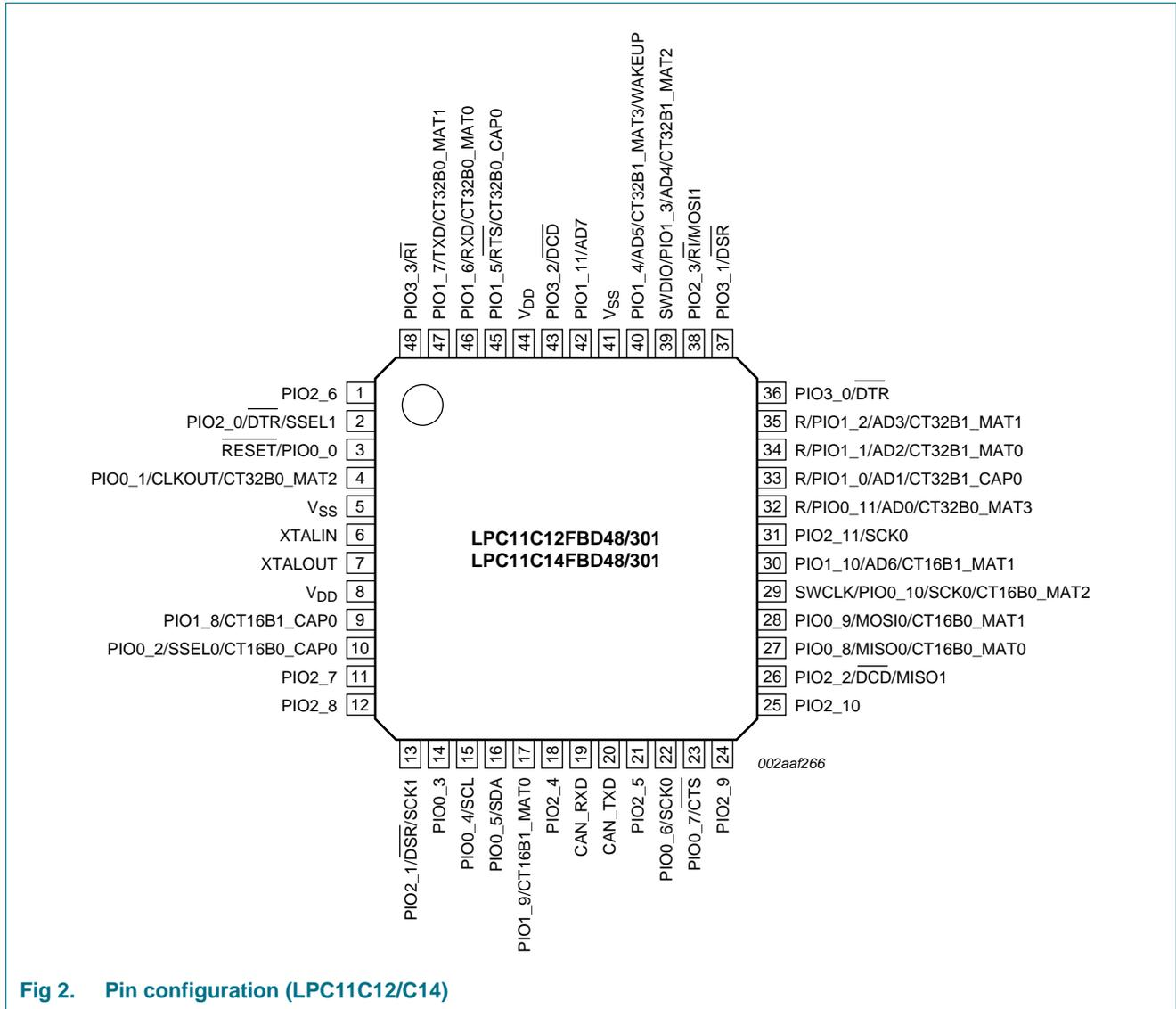
Fig 2. Pin configuration (LPC11C12/C14)
