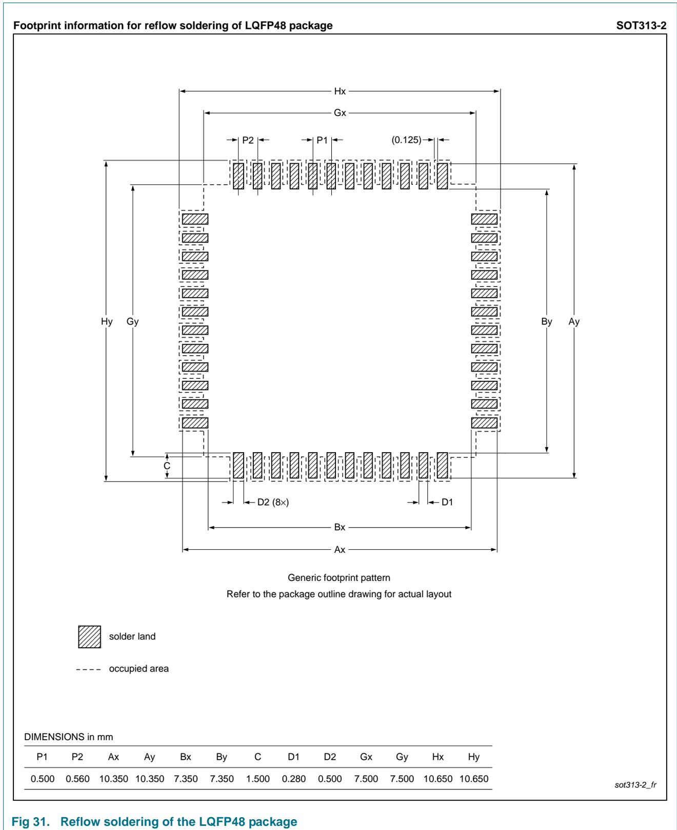
Fig 31. Reflow soldering of the LQFP48 package
