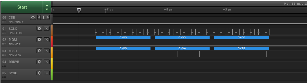
Figure 40. A1 is measured at last falling edge of SPI clock, A2 is measured at falling edge of DRDYB pin
