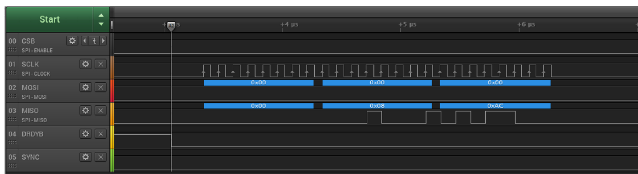
Figure 43. A1 is measured at rising edge of SYNC pulse, A2 is measured at falling edge of DRDYB pin
