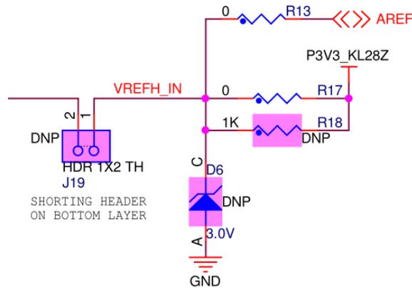
Figure 14. VREFH circuit schematic
