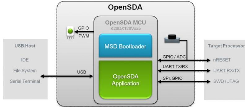
Figure 4. OpenSDA block diagram
