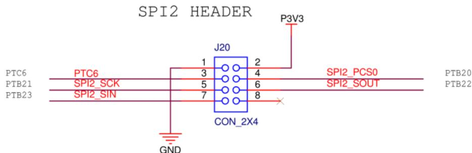
**Figure 13. Header SPI2 Header****Table 9. SPI2 Header connections**
