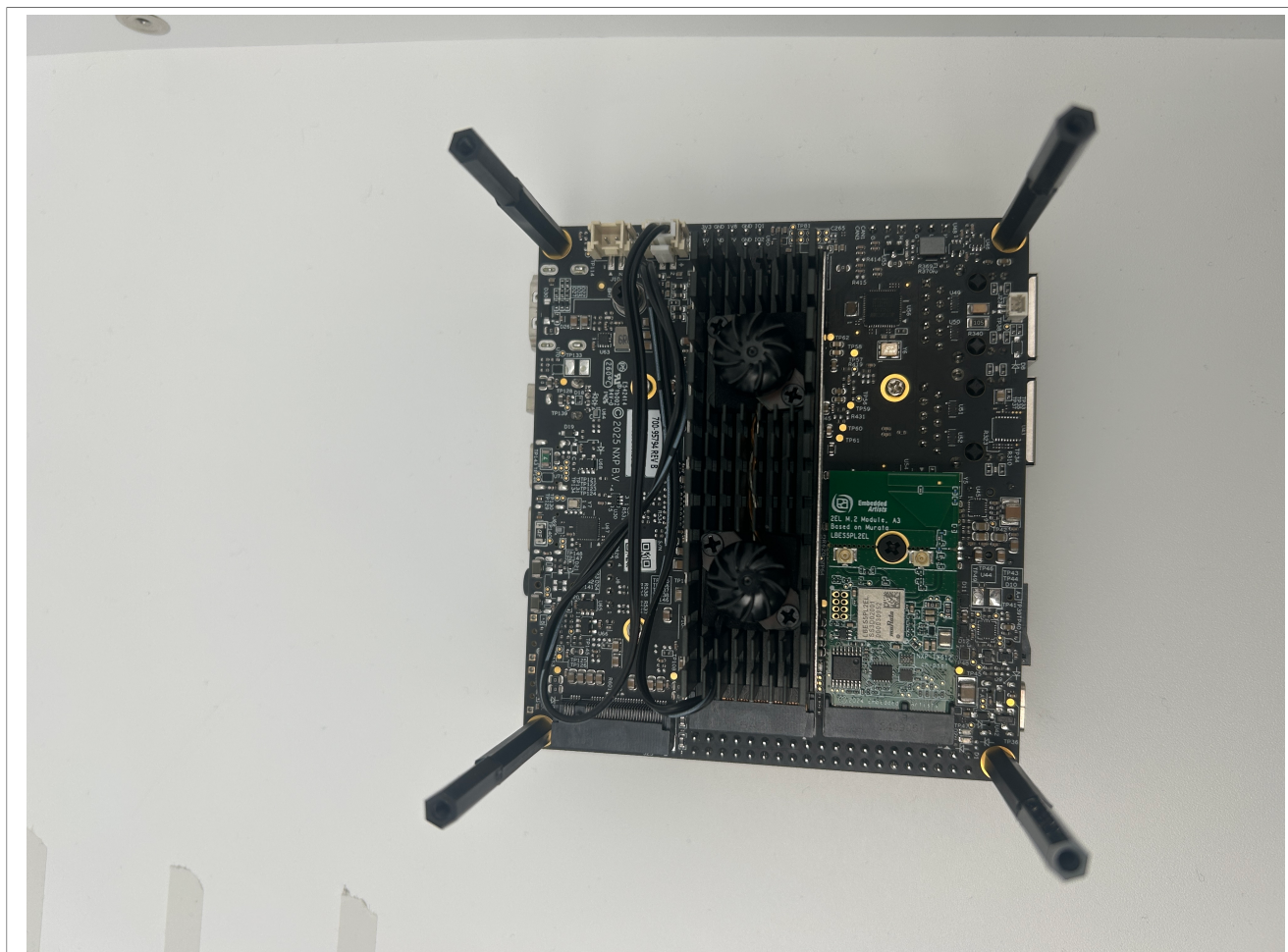
Figure 8. ARA2-M2-16G-GT to FRDM-IMX95-PRO connection — Front view
