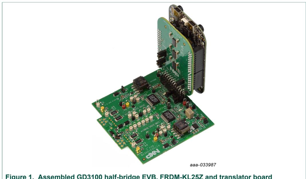
Figure 1. Assembled GD3100 half-bridge EVB, FRDM-KL25Z and translator board
