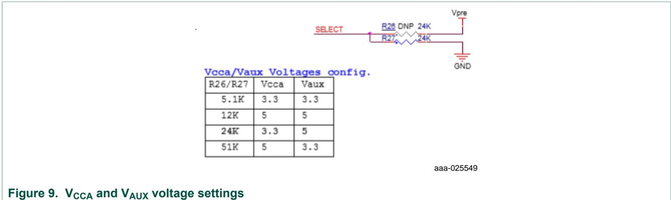
Figure 9.  $V_{CCA}$  and  $V_{AUX}$  voltage settings
