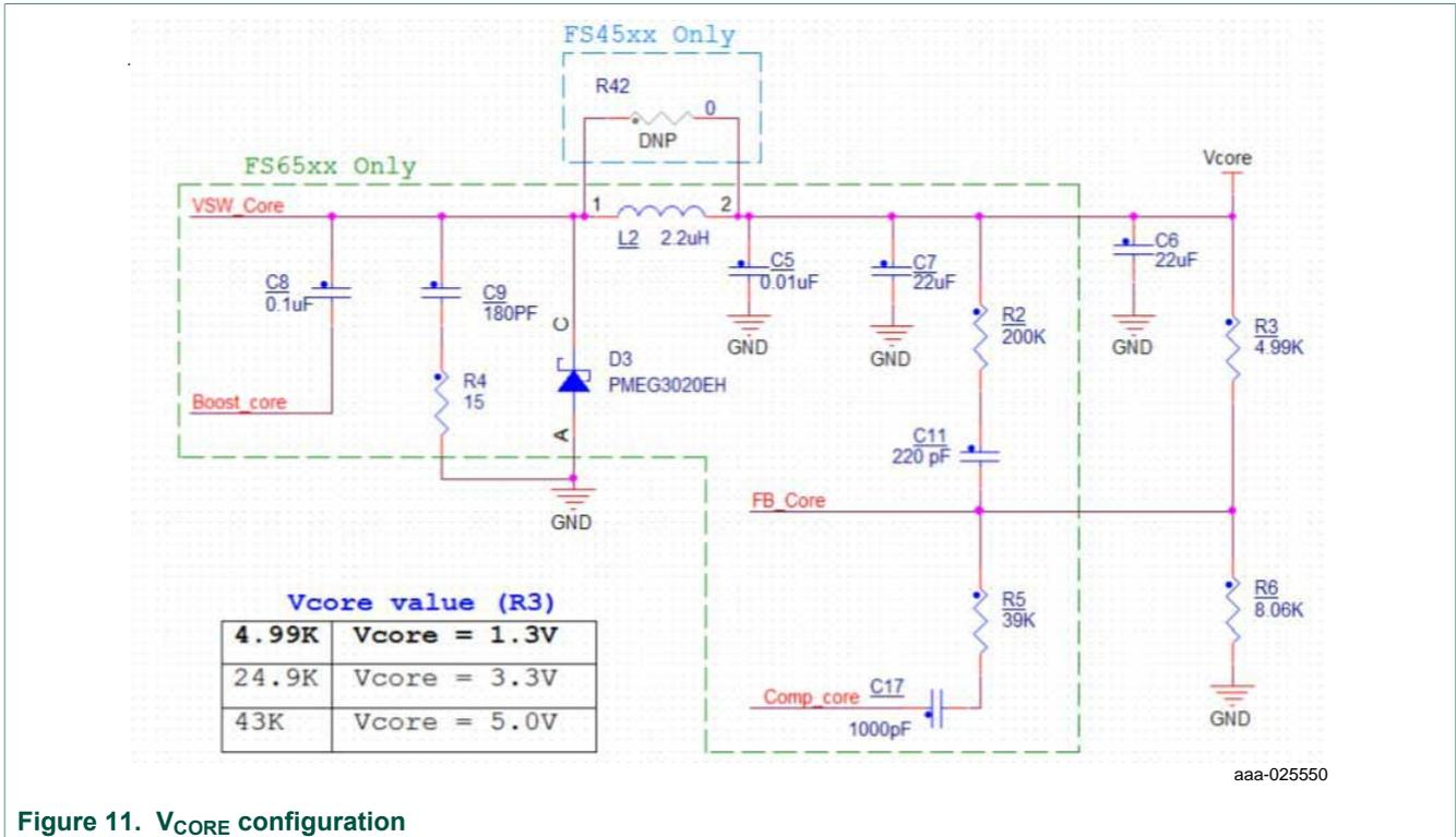
Figure 11. V<sub>CORE</sub> configuration
