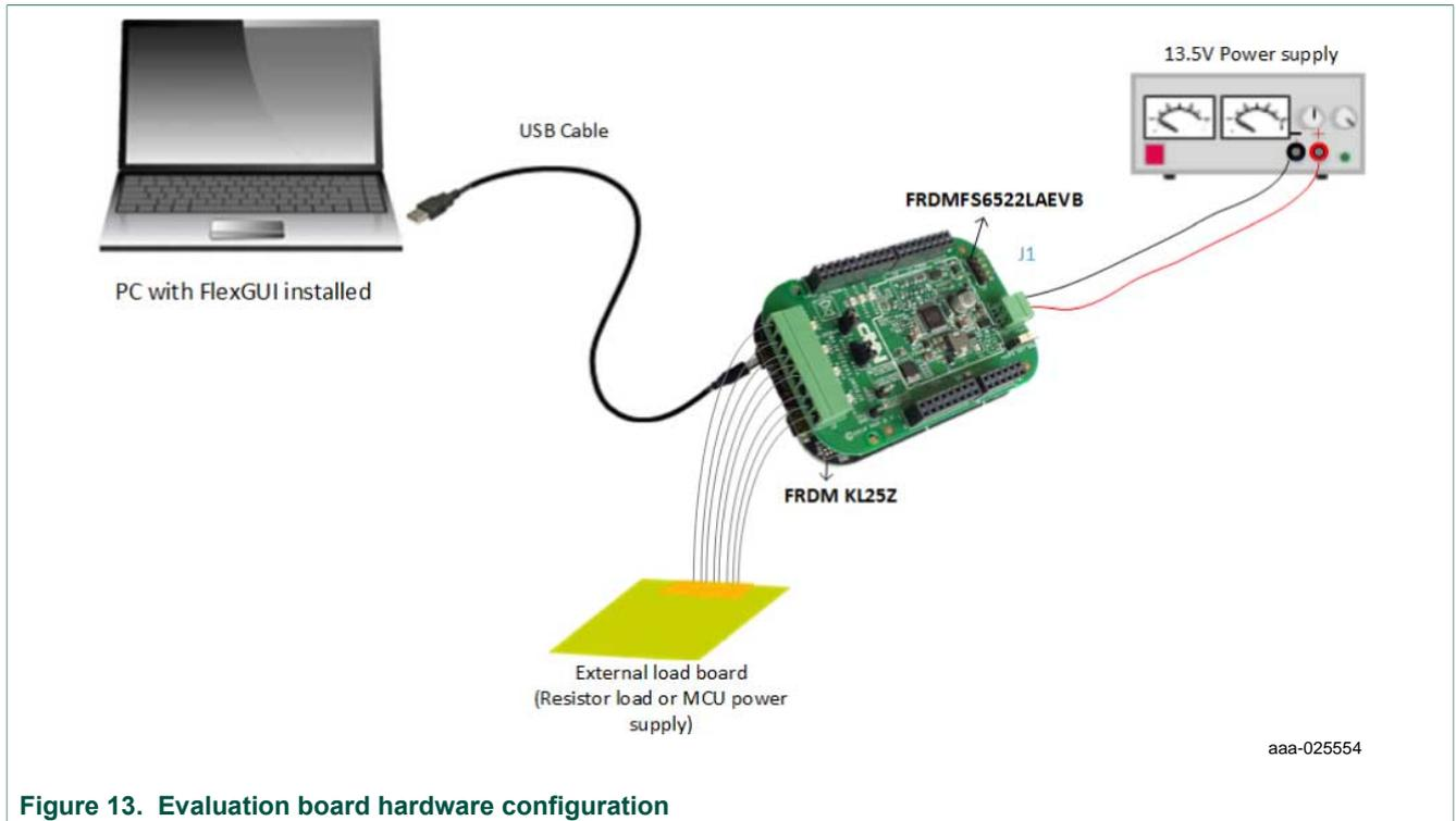
**Figure 13. Evaluation board hardware configuration**
