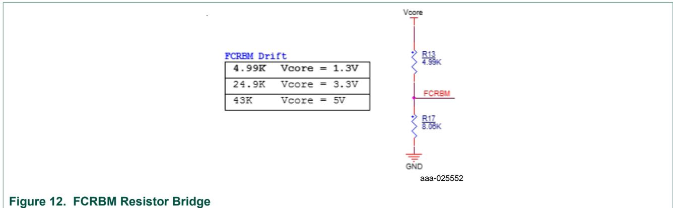
Figure 12. FCRBM Resistor Bridge
