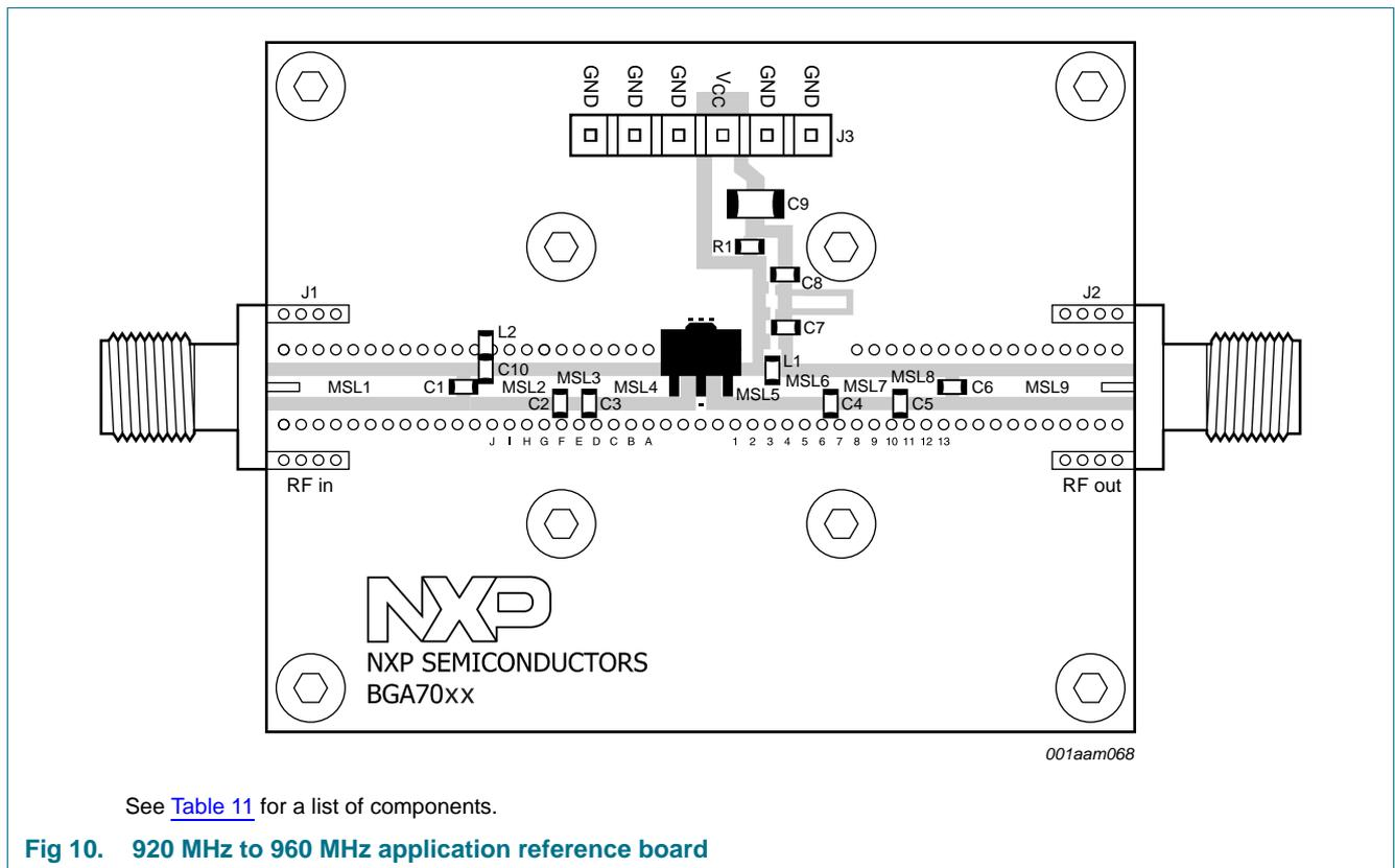
**Table 11. List of components of 920 MHz to 960 MHz**See [Figure 2](#) and [Figure 10](#) for component layout.Printed-Circuit Board (PCB): Rogers RO4003C stack; height = 0.508 mm; copper plating thickness = 35  $\mu$ m.
