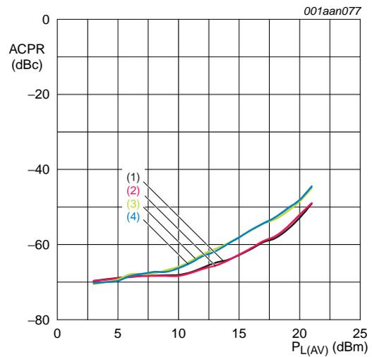
2-carrier W-CDMA; each carrier according to 3GPP test model 1; 64 DPCH; PAR for composite signal = 9 dB; 10 MHz carrier spacing.
