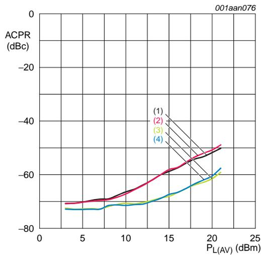
2-carrier W-CDMA; each carrier according to 3GPP test model 1; 64 DPCH; PAR for composite signal = 7.5 dB; 5 MHz carrier spacing.
