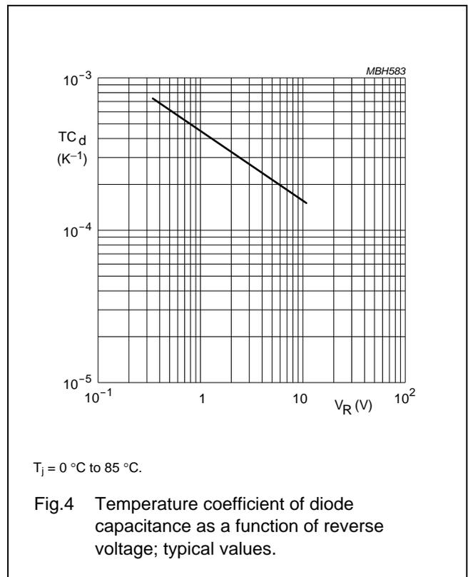
Low-voltage variable capacitance diode
