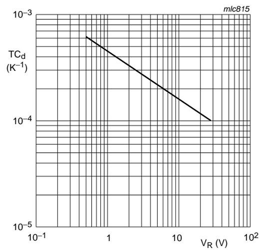
$T_j = 0 \text{ }^\circ\text{C} \text{ to } 85 \text{ }^\circ\text{C}.$
