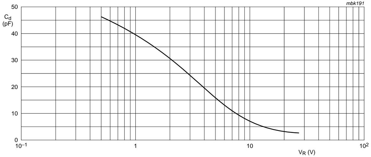
$f = 1 \text{ MHz}; T_j = 25 \text{ }^\circ\text{C}.$
