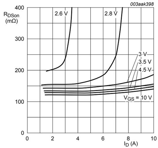
$$T_j = 25^\circ\text{C}; t_p = 300 \mu\text{s}$$
