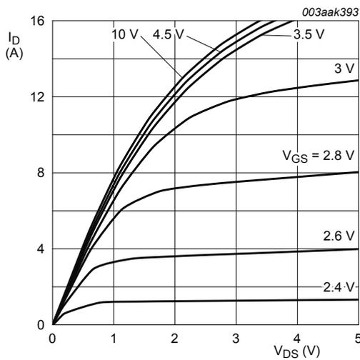
$T_j = 25\text{ °C}; t_p = 300\text{ }\mu\text{s}$
