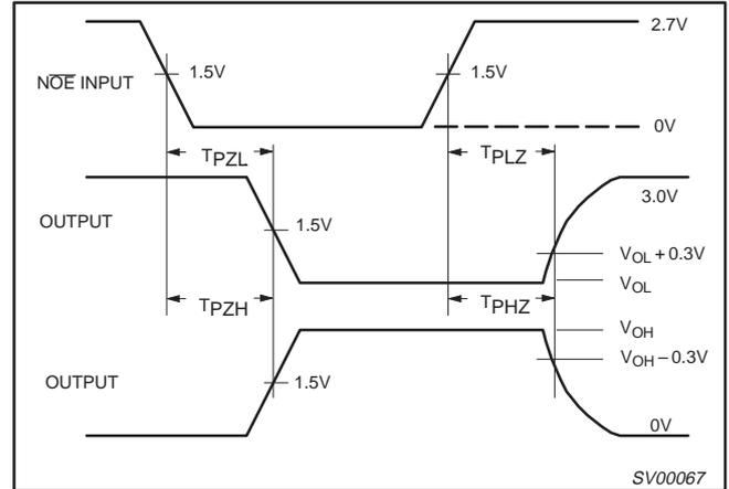
Waveform 2. 3-State Output Enable and Disable Times
