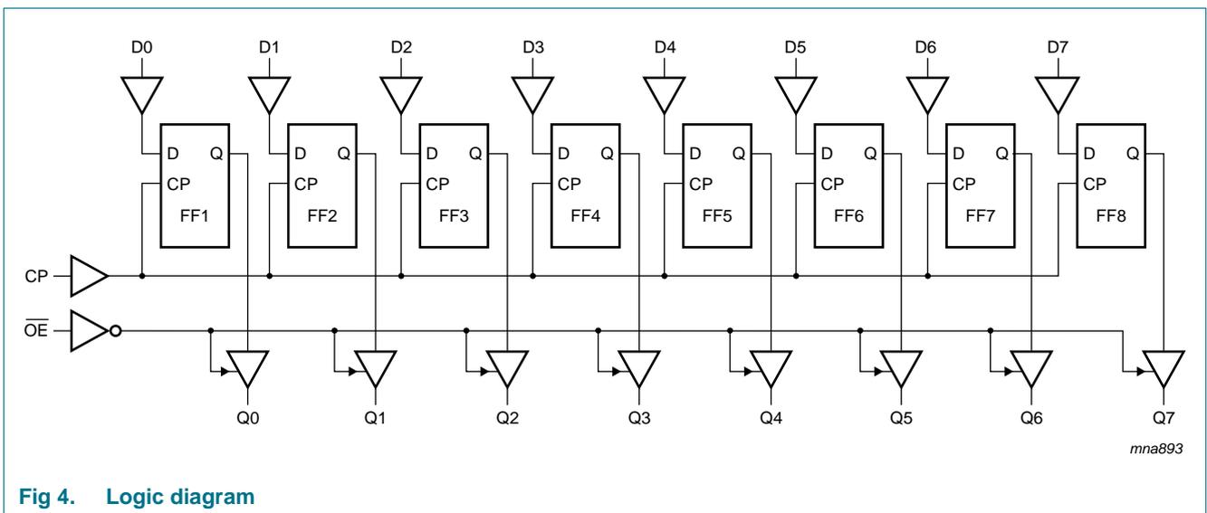
**Fig 4. Logic diagram**
