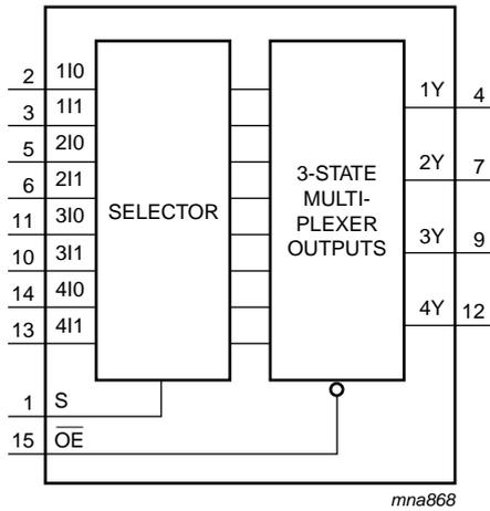
Fig 3. Functional diagram
