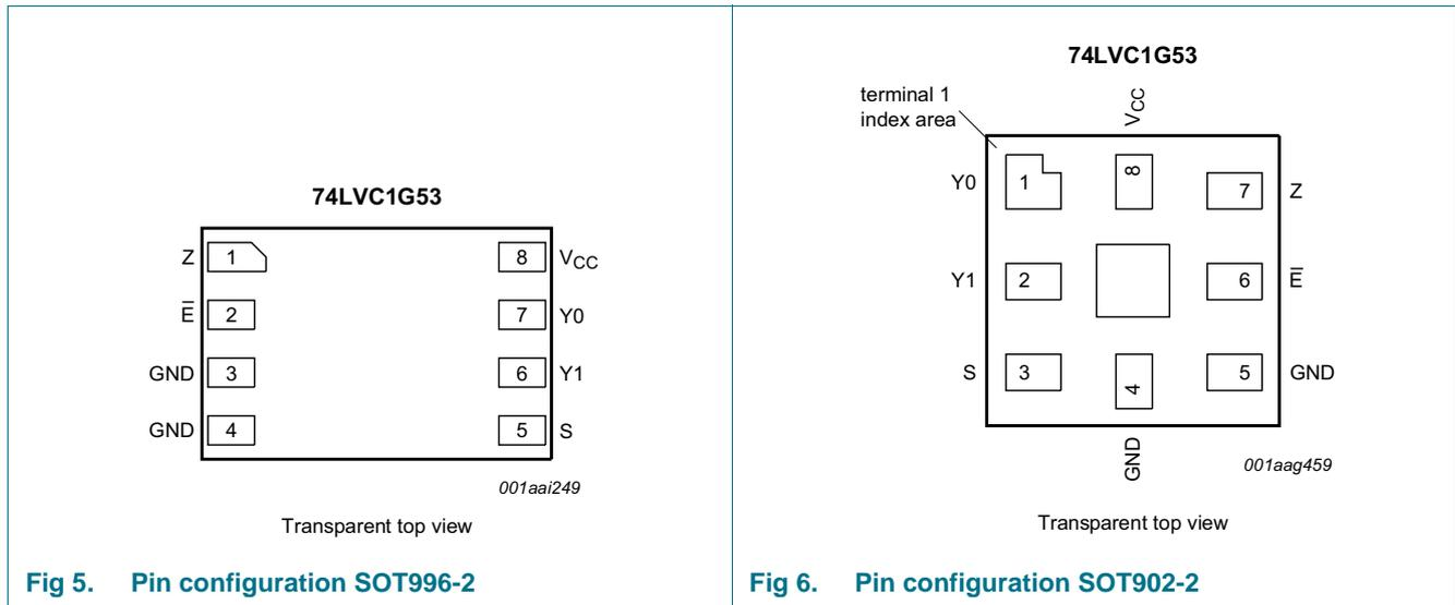
Fig 5. Pin configuration SOT996-2
