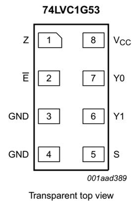
Fig 4. Pin configuration SOT833-1, SOT1089, SOT1116 and SOT1203
