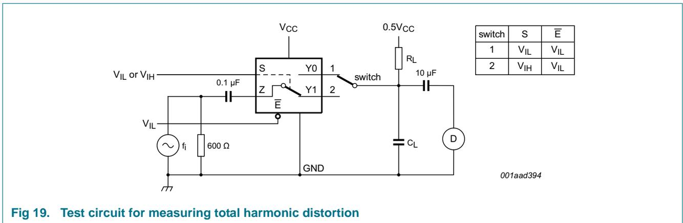
**Fig 19. Test circuit for measuring total harmonic distortion**
