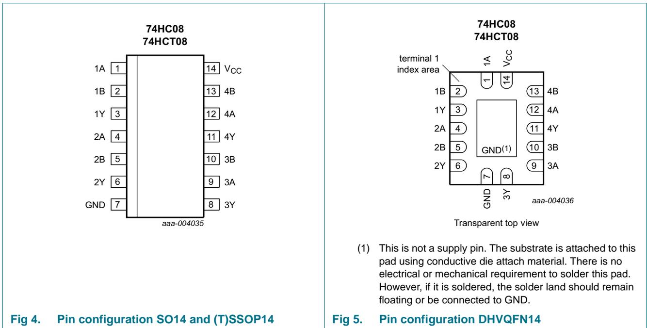
(1) This is not a supply pin. The substrate is attached to this pad using conductive die attach material. There is no electrical or mechanical requirement to solder this pad. However, if it is soldered, the solder land should remain floating or be connected to GND.
