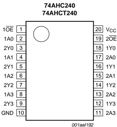
Fig 3. Pin configuration SO20 and TSSOP20
