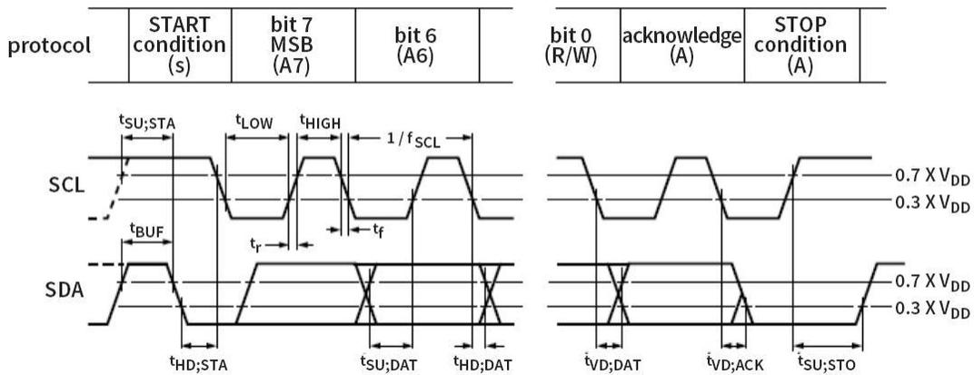
Figure 5.3 I<sup>2</sup>C-bus timing diagram
