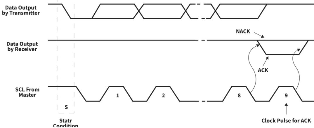
Figure 6.5 Acknowledgment on the I<sup>2</sup>C Bus
