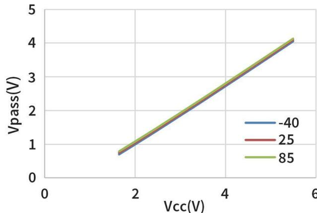
Figure 7.2 Pass-Gate Voltage (V<sub>pass</sub>) vs Supply Voltage (V<sub>CC</sub>) at Three Temperature Points
