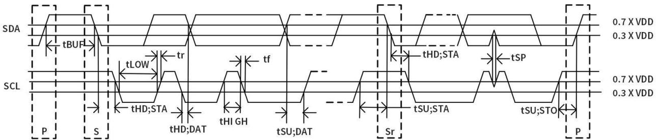
Figure 5.1 Definition of timing on I<sup>2</sup>C-bus
