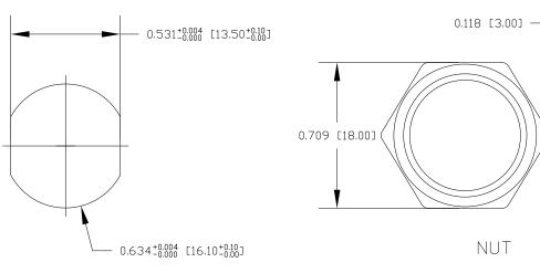
NOTE: MATERIAL HOUSING: CONTACT: NUT: SHELL: □-RING: FINISH CONTACT: UNDER PLATE: ELECTRICAL RATED CURRENT: M16×1.5 RATED VOLTAGE: INSULATION RESISTANCE: CONTACT RESISTANCE: WATER PROOF: ENVIRONMENT OPERATION TEMPERATURE: -40°C ~ +85°C
