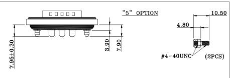
NOTE: MATERIAL HOUSING PBT UL94V-0, BLACK **FLANGE** PBT UL94V-0, BLACK CONTACT BRASS, PLATING P/N KEY BELOW STEEL, NICKEL SHELL O-RING SILICONE SEALING COMPOUND **EPOXY** HARDWARE BRASS; NICKEL PLATED ELECTRICAL POWER CONTACT RATED CURRENT P/N KEY BELOW VOLTAGE 1000 VAC 1 MIN INSULATOR RESISTANCE 5 G0hms MIN. POWER CONTACT RESISTANCE 1.0 m0hms MAX. WATER PROOF IP67 ENVIRONMENT OPERATION TEMPERATURE -25°C TO +85°C
