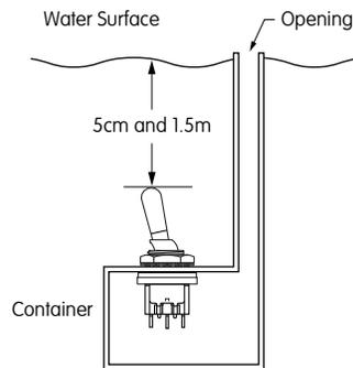
Repeat opening and closing same as previous test. The resulting insulation resistance and voltage capacity are both within the rated values, and water has not entered inside the switch or installation panel.
