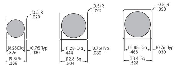
**Film Insert Material and Thickness:** Clear Polyester; 4 mil (100μ) maximum thickness
