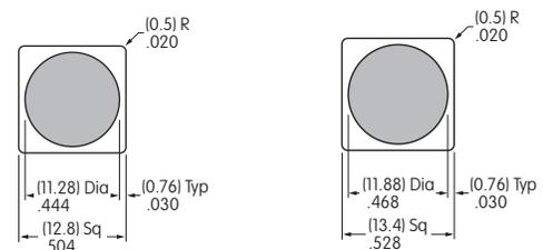
Film Insert Material and Thickness: Clear Polyester; 4 mil (100µ) maximum thickness
