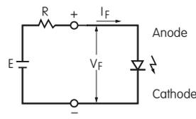
$R = \frac{E - V_F}{I_F}$ <p>Where: R = Resistor Value (Ohms)<br/>                     E = Source Voltage (V)<br/>                     V<sub>F</sub> = Forward Voltage (V)<br/>                     I<sub>F</sub> = Forward Current (A)</p> |
