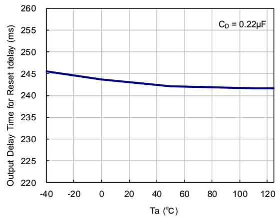
18) Detect Output Delay Time vs. Temperature
