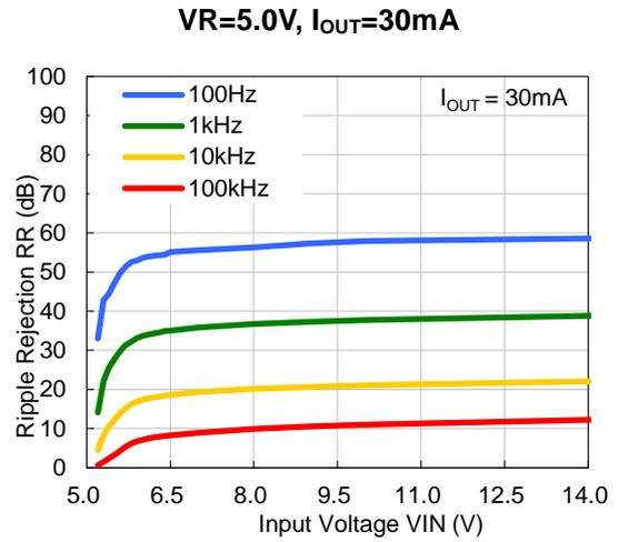
10) Ripple Rejection vs. Frequency (Ta=25°C, Ripple=0.2 Vpp)
