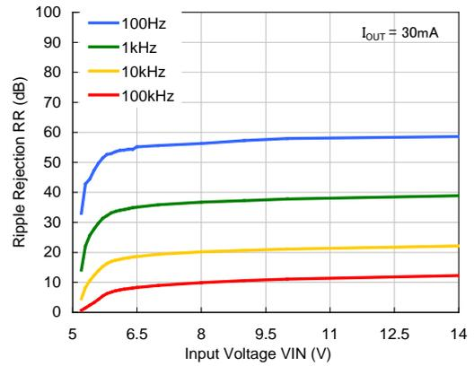
10) Ripple Rejection vs. Frequency (Ta=25°C, Ripple=0.2 Vpp)
