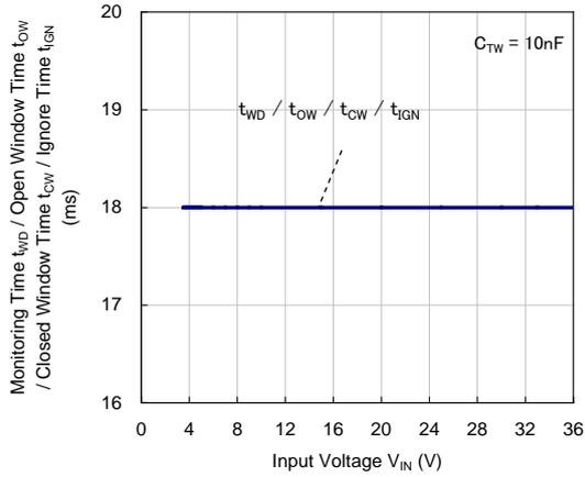
21) Reset Time vs. Input Voltage
