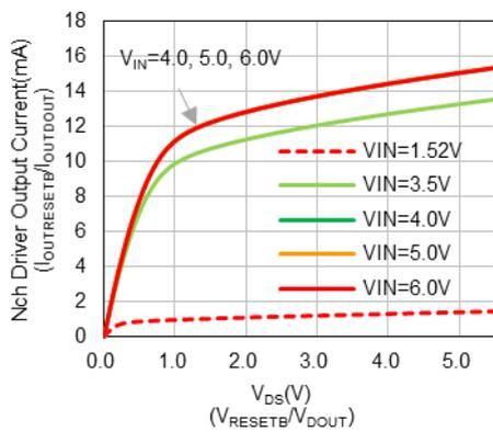
28) Nch. Driver Output Current vs. Input Voltage
