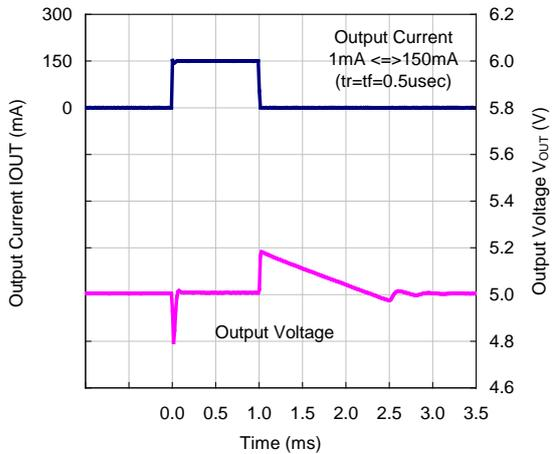
13) CE Transient Response ( $T_a=25^{\circ}\text{C}$ ,  $V_{IN}=14\text{V}$ ,  $I_{OUT}=1\text{mA}$ ,  $C_{OUT}=0.1\mu\sim 47\mu\text{F}$ )
