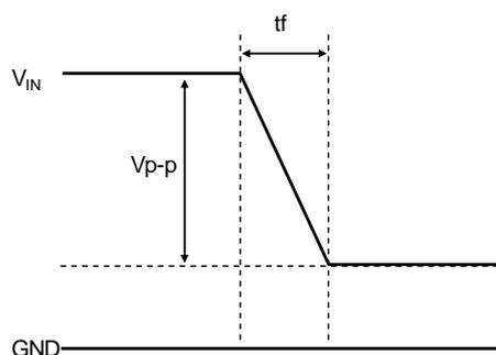
Prohibited Area of Fluctuation at Falling of  $V_{IN}$
