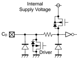
**<RESETB pin(R5110Sxx1x) / D<sub>OUT</sub> pin(R5110xxx2x)>**
