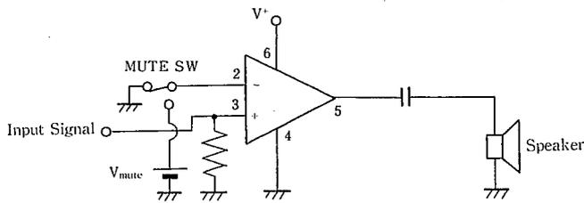
According to this method, when applying DC voltage,  $V_{mute}$  to -INPUT PIN, the output voltage  $V_o$  at voltage gain  $A_v$  will be,
