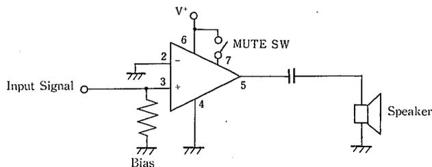
By this way, the bias circuit within IC, to be stopped and then, further for stopping motion of driver level, and at the output level. However, the input level alone is operating, so that a slight leakage of signal to the output pin through inside resistor to be occurred. The leakage level is to be inverse proportion to load, therefore, it is necessary to check accordingly through the load condition.
